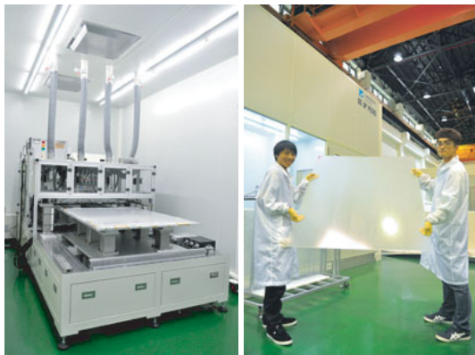
Figure 1 Demonstrator aePLASMA coating machine, left, capable of handling fifth-generation, 1,100 × 1,400 mm, large-size glass plate.
