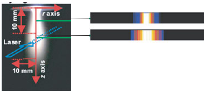
Figure 6 Measuring the temperature in an aePLASMA atmospheric environment plasma jet stream using a digital camera. Laser-induced fluorescence (LIF) technique is used in this measurement. The top ICCD camera image at right shows the LIF image of a plasma jet of NO at 5 mm down stream the nozzle exit, and left image at right shows the LIF of the jet at about 11 mm down stream.
