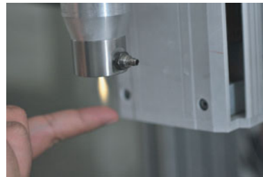
Figure 3 ITRI aePLASMA is low-temperature plasma technology. Temperature of the plasma jet lowers to room temperature about a few millimeters (8 mm) from the exit of the nozzle.
