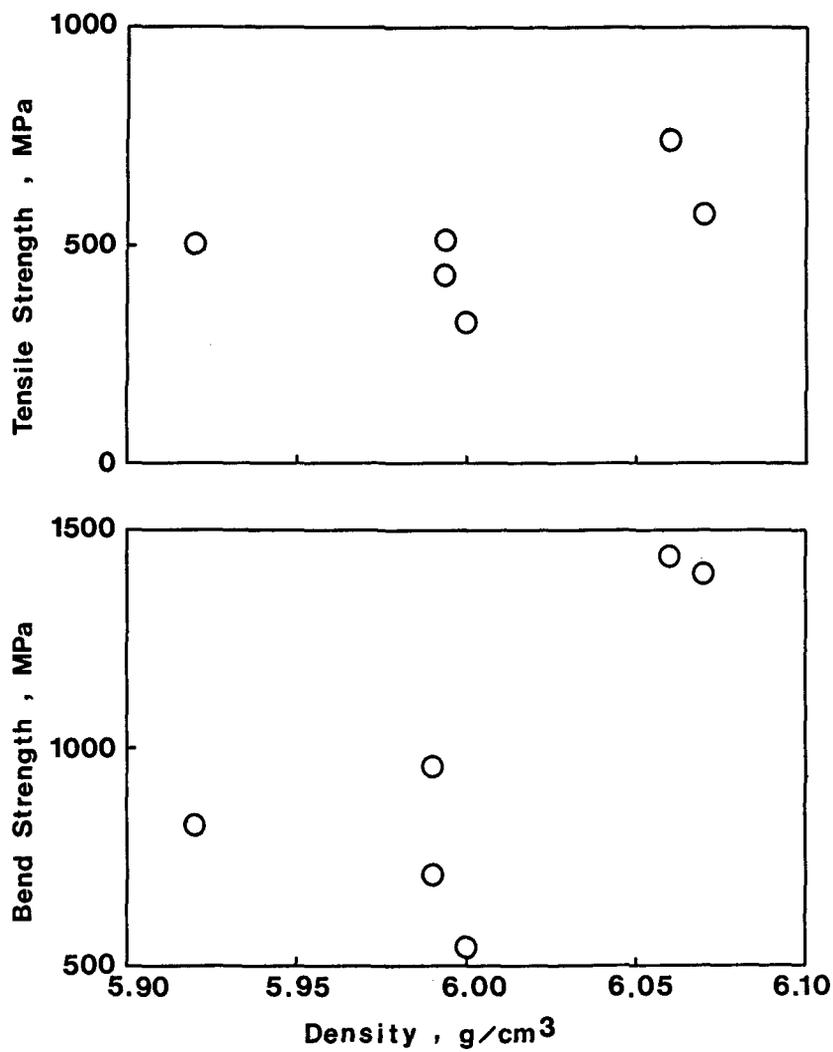
Figure 1. Plot of bulk density vs. strength of Y-TZP
