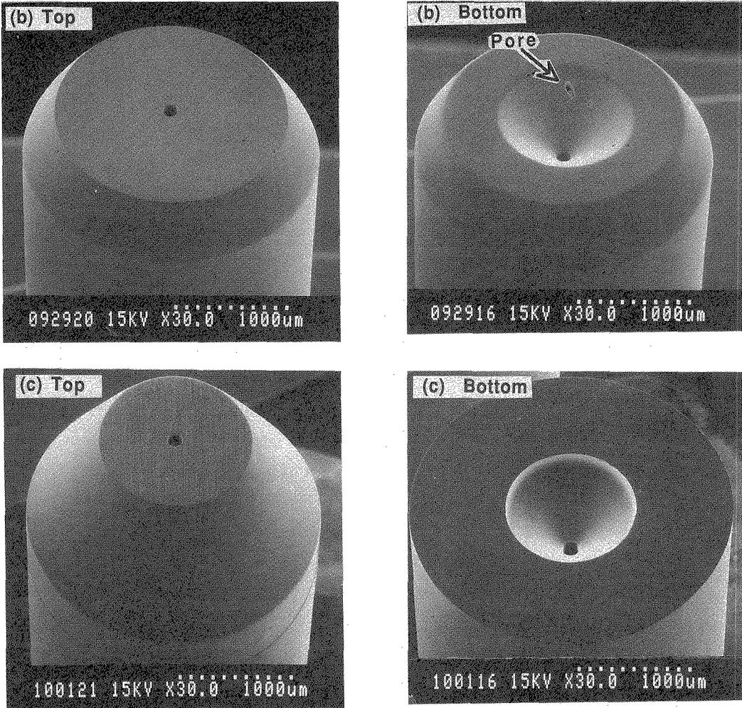
Figure 13. SEM photographs of PSZ ferrules obtained by the conventional process (b) and the sintered sample obtained by the present process (c).
