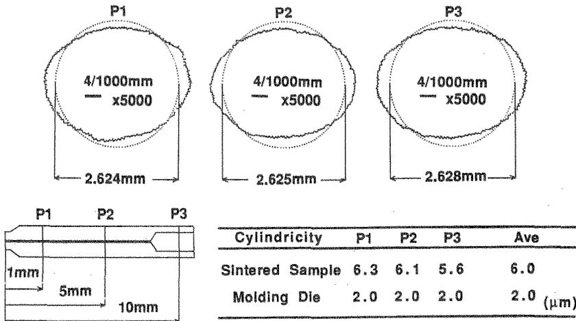
Figure 12. Cylindricity measurement results of a PSZ ferrule.
