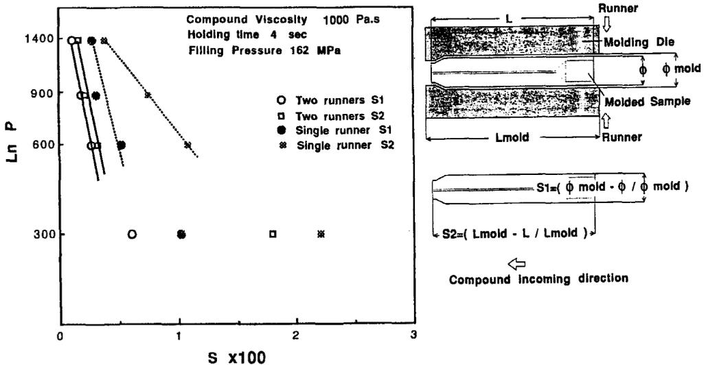
Figure 4. Relationship between the sample dimensions,  $\phi$  and  $L$ , and die dimensions,  $\phi_{mold}$  and  $L_{mold}$ , and the holding pressure.
