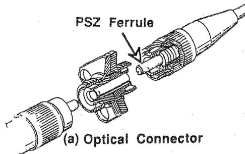
Figure 13. Schematic diagram of optical connector (a)
