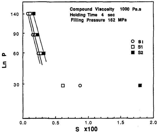
Figure 8. Relationship between the holding pressure and the line shrinkage  $S_\ell$  obtained by Archimedes's method, and  $S_1$  and  $S_2$  obtained by measurement of the dimensions of the molded samples.
