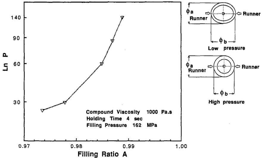
Figure 5. Relationship between the holding pressure and the filling ratio,  $A$ .
