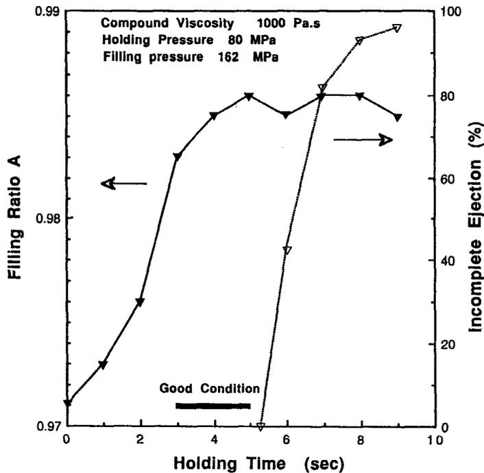
Figure 9. Relationship between the duration of holding pressure and the filling ratio,  $A$ , and the percentage of incomplete mold ejection.
