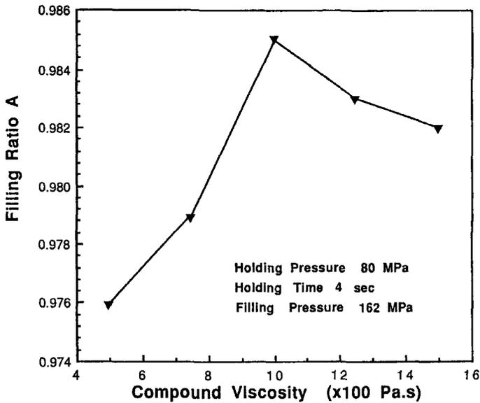
Figure 10. Relationship between the viscosity of the compound and the filling ratio, A.
