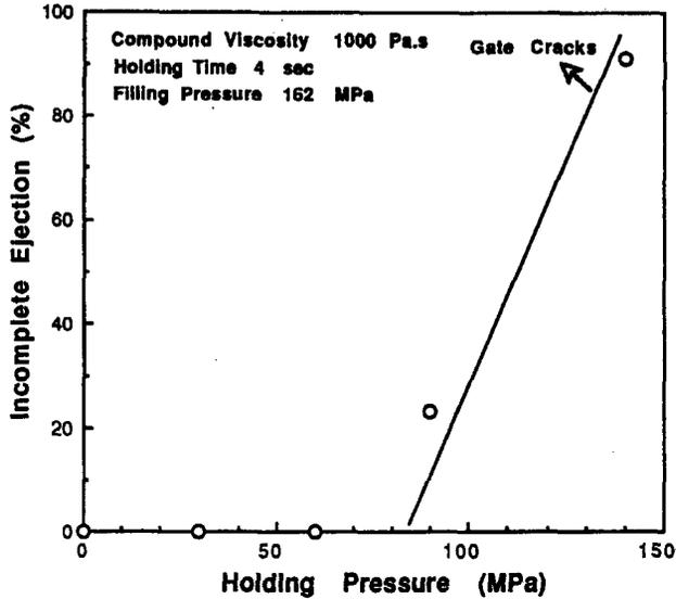
Figure 6. Relationship between the holding pressure and the percentage of incomplete mold ejection.
