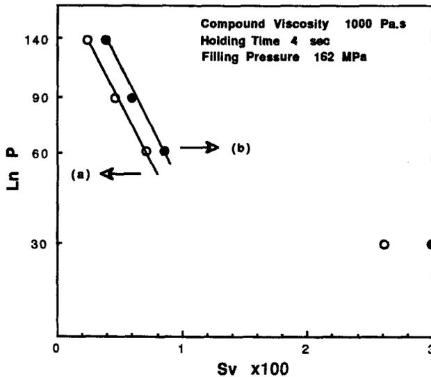
Figure 7. Relationship between the holding pressure and the volumetric shrinkage ratio.
