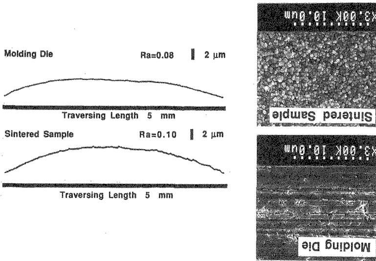
Figure 11. Surface roughness and SEM photograph of the molding die and of the sintered sample.
