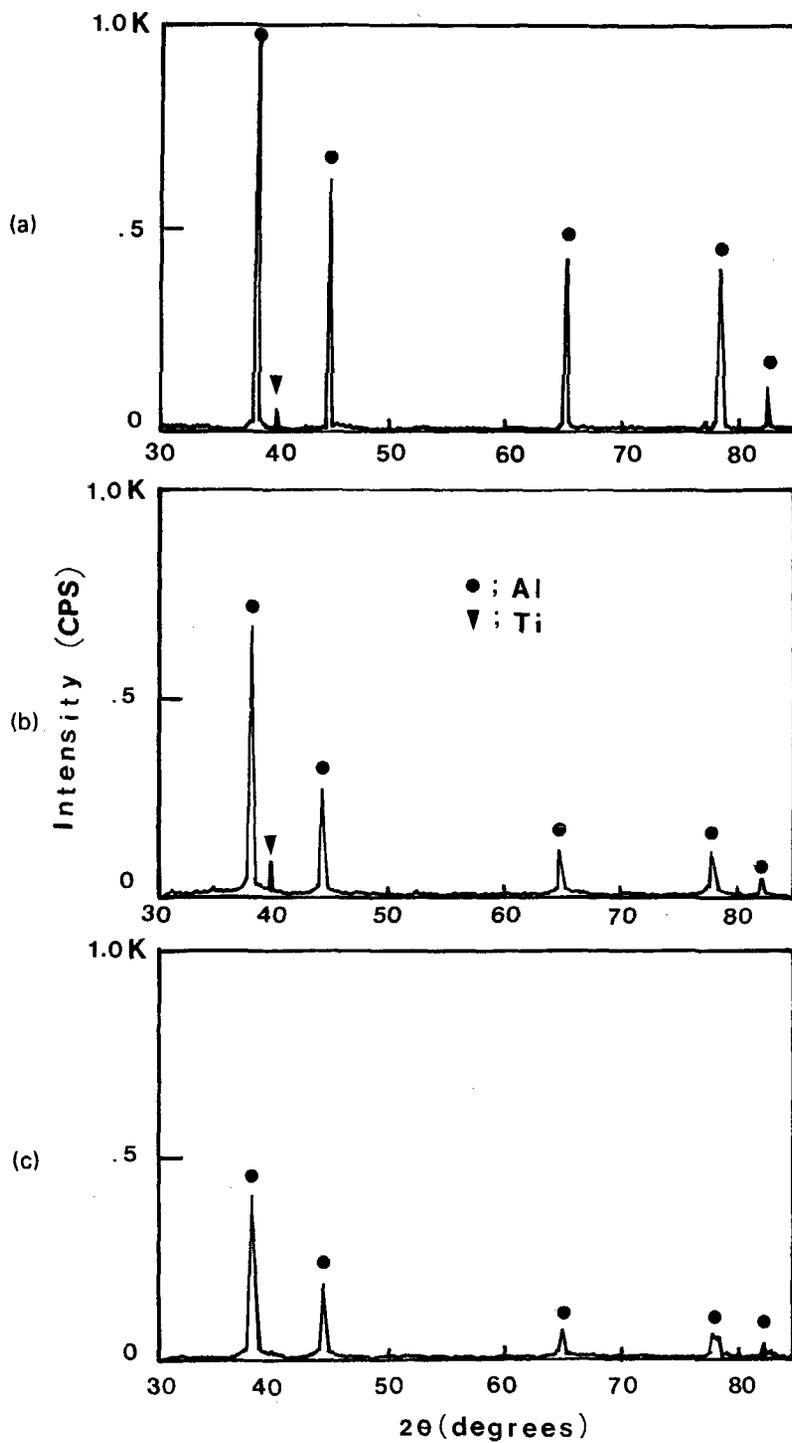
Figure 7. X-ray diffraction patterns of MA Al-8wt.%Ti powders after mechanical alloying for (a) just blended, (b) as-attrited for 10hr. and (c) for 15 hr.
