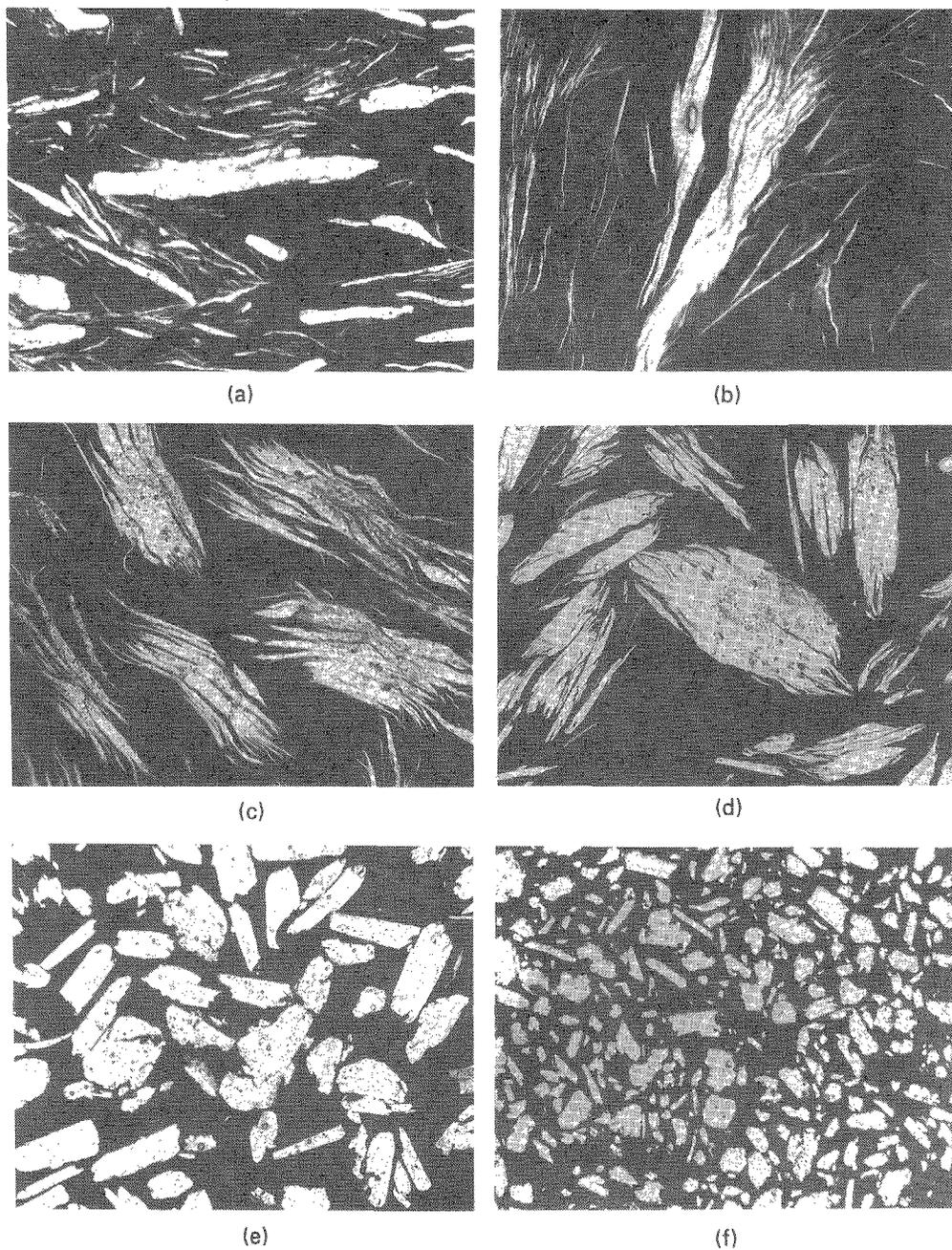
Figure 2. Optical micrographs of mechanically alloyed powder processed for various times; (a) 30min., (b) 1hr., (c) 2hr., (d) 3hr., (e) 7hr. and (f) 15hr.
