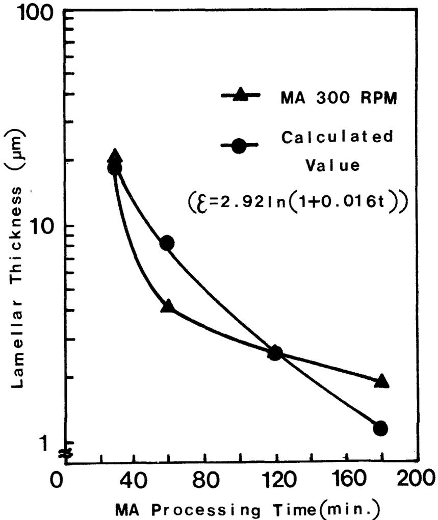
Figure 4. Variation of lamellar thickness as a function of MA processing time.
