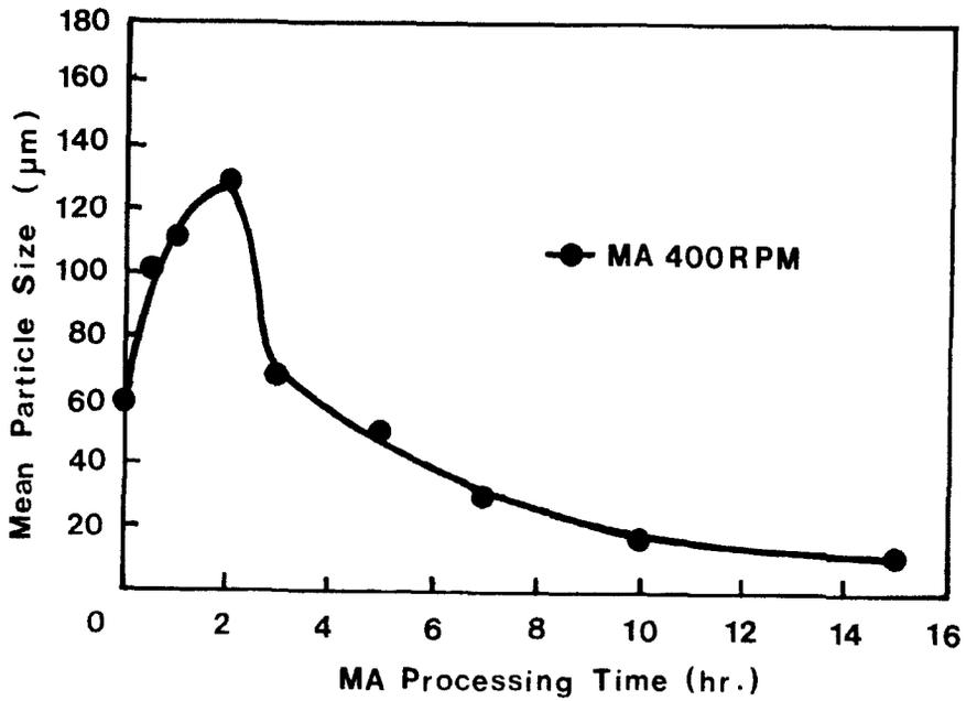
Figure 5. The relation between mean particle size and MA processing time with milling speed of 400rpm.
