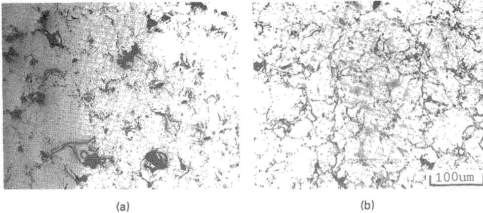
Figure 10. Optical micrographs of MA Al-8wt.%Ti powder compact; (a) sintered at 600°C in N<sub>2</sub> atm. for 1hr. after cold pressing (88% T.D.) and (b) hot pressed in a vacuum of  $1 \times 10^{-2}$  torr at 430°C for 1 hr. (98% T.D.)
