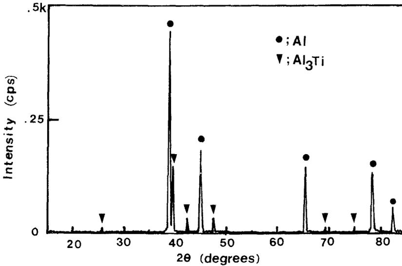
Figure 11. X-ray diffraction pattern of MA Al-8wt.%Ti powder compact, hot pressed in a vacuum of  $1 \times 10^{-2}$  torr at 430°C for 1hr.
