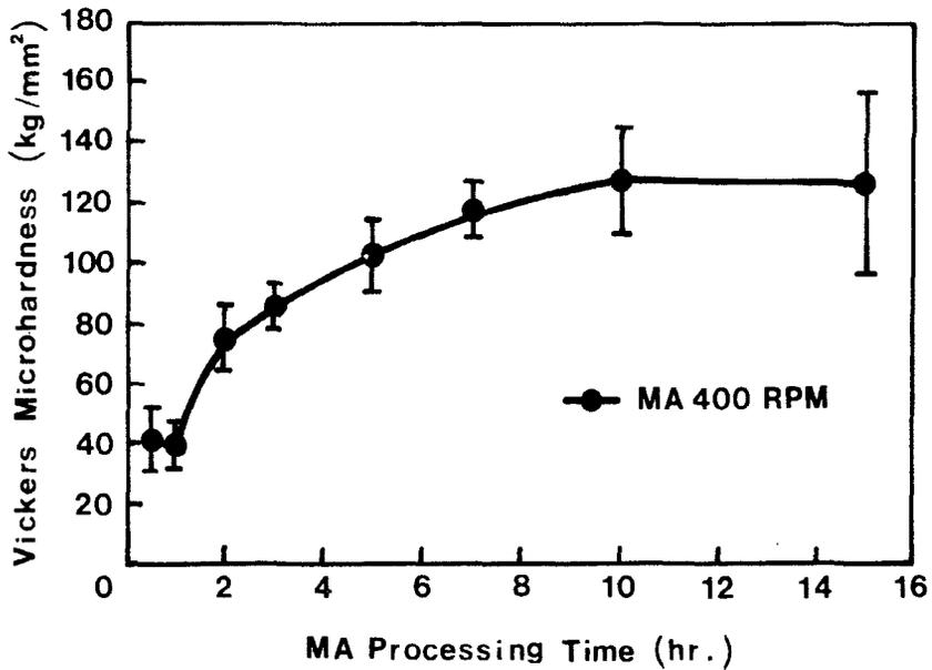
Figure 6. Variation of microhardness as a function of milling times in mechanical alloying of the Al-8wt.%Ti powder.
