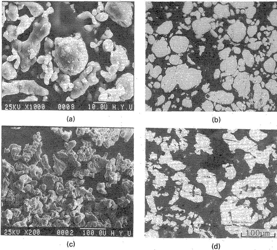
Figure 1. SEM morphologies(a,c) and optical micrographs(b,d) of elemental powder used in the present study; Al powder(a,b) and Ti powder(c,d)
