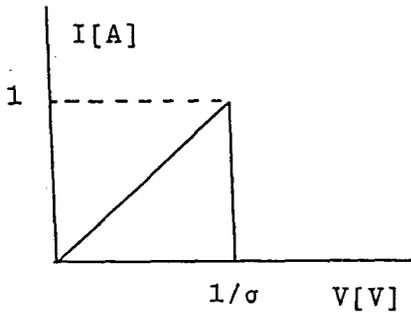
Fig.1. I-V characteristic for a single fuse. Above a current of 1[A], no current flows.
