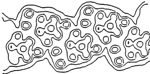
Fig. 3 is the grain boundary structure with tensile stress perpendicular to the grain boundary. The stress applied was  $1 \times 10^3$  MPa. Initially crack path was set on the grain boundary plane inside the structure unit at the both sides. After the stress was applied the fracture path was along the side of the structure units expected as the weaker bond region by the molecular orbital calculations.
