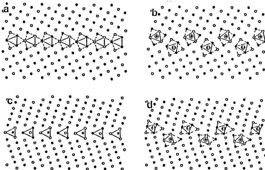
Fig. 1 Grain boundary structures of  $\Sigma=5$  (a,b) and  $\Sigma=9$  (c,d) coincidence grain boundaries without P (a,c) and with P segregation (b,d). Double circles indicate P atom positions. Black and white circles indicate the different atom planes.
