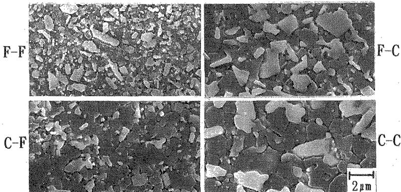
Fig.1 Microstructure of  $\text{Al}_2\text{O}_3$ -30%TiC specimen, after thermal etching.
