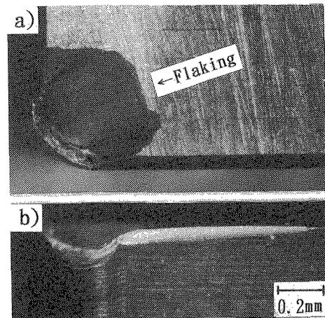
Fig. 2 An example of flaking (indicated by arrow) occurring parallel to the crater surface. a) crater surface, b) flank surface.
