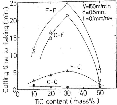
Fig. 3 Effects of TiC content and grain size of  $Al_2O_3$ -TiC ceramics tools on cutting time to flaking in turning test of SKD11.
