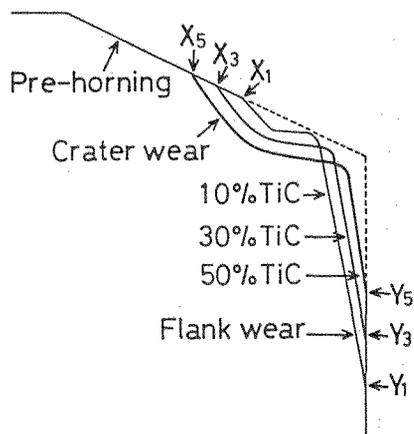
Fig. 5 Schematic drawing of crater and flank surface of  $Al_2O_3$ -TiC(F-F) ceramics tools in turning test for 20min.  $V=150$ m/min,  $d=0.5$ mm,  $f=0.1$ mm/rev, coolant, not used.
