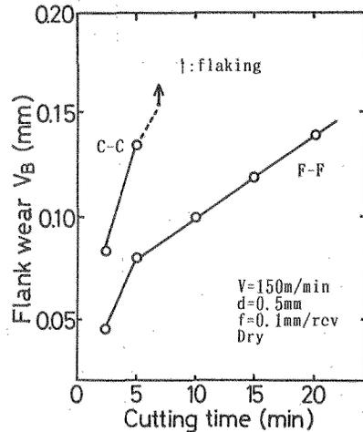
Fig. 4 Effect of grain size of  $Al_2O_3$ -30%TiC ceramics tools on flank wear in turning test of alloyed tool steel.
