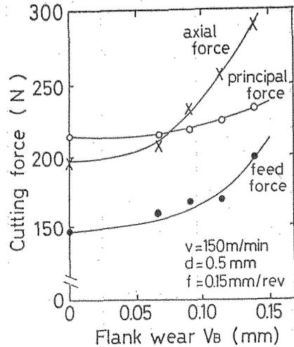
Fig. 7 Relation between cutting force and flank wear ( $V_B$ ).  $Al_2O_3$ -30%TiC (F-F) commercialized tool is used.
