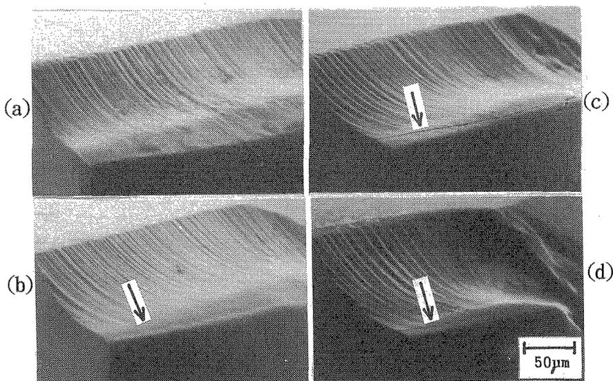
Fig. 6 Crater wear of  $Al_2O_3$ -30%TiC(F-F) ceramics tool in turning test of SKD11 for 5-20min. An arrow shows crack formation on crater surface. Cutting condition, the same as Fig. 3. a) 5min, b) 10min, c) 15min, d) 20min.
