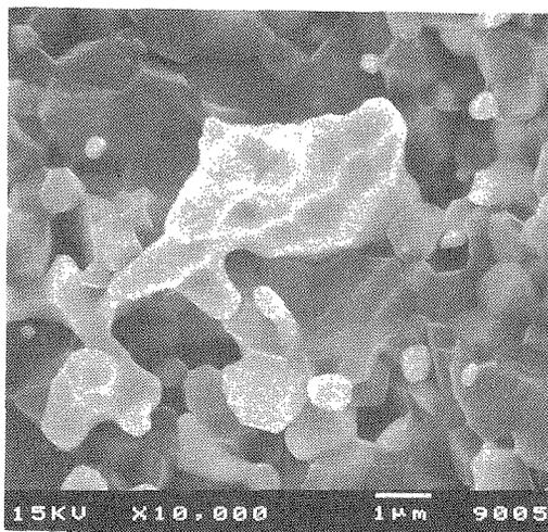
Fig.1 Scanning electron micrograph on the fracture surface of  $\text{Al}_2\text{O}_3$  composite dispersed by the ball milling method. Largest Pd-particle size is about  $5 \mu\text{m}$ .
