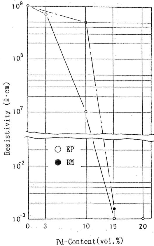
Fig.9 Resistivity vs. Pd content of composites.
