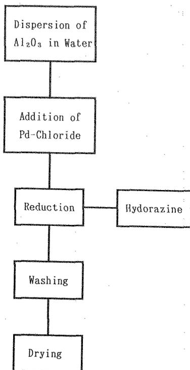
Fig.2 Process of Pd electroless plating on  $\text{Al}_2\text{O}_3$  powders.
