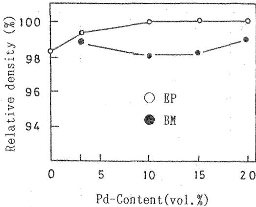
Fig. 4 Relative density vs. Pd content of composites.
