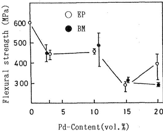
Fig. 6 Flexural strength Pd content of composites.
