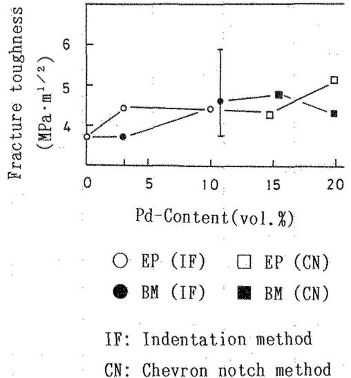
Fig. 7 Fracture toughness vs. Pd content of composites.
