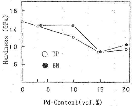
Fig. 5 Hardness vs. Pd content of composites.
