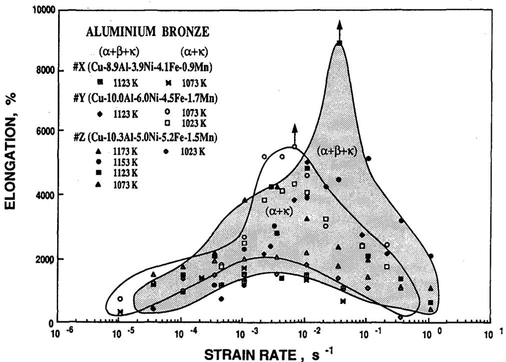
Figure 4. The superplastic elongations of three aluminum bronzes #X, #Y and #Z as a function of strain rate for different temperatures between 1023 and 1173 K, at which these alloys have complex microstructures consisting of  $\alpha+\gamma$  or  $\alpha+\beta+\gamma$  phases.
