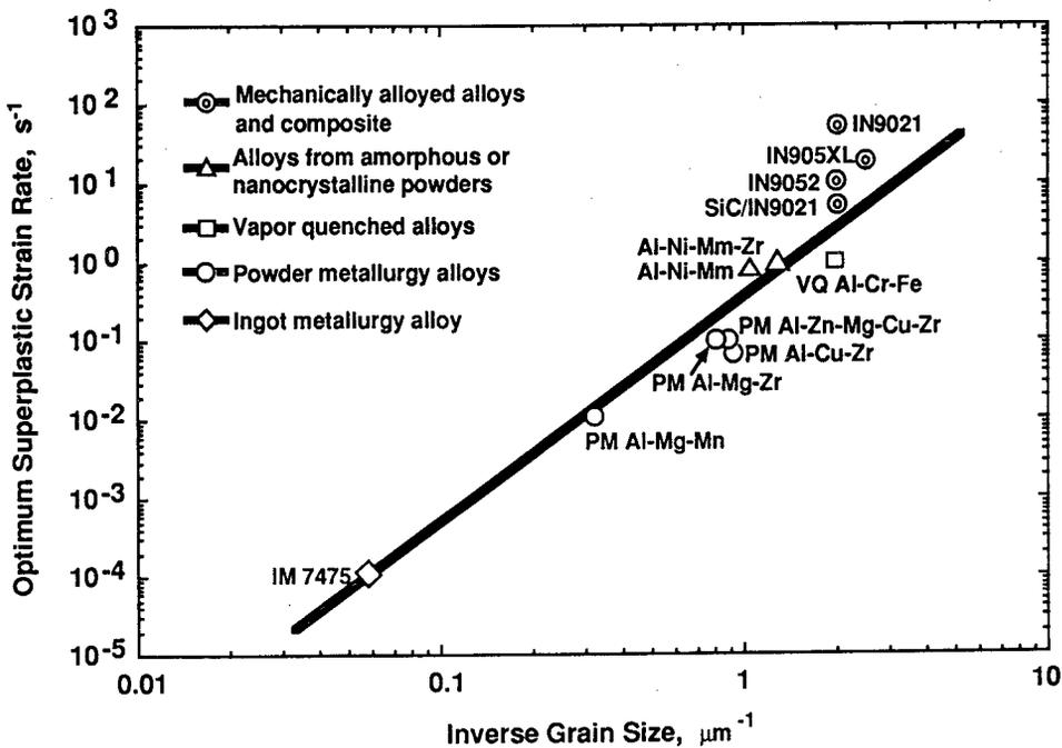
Figure 9. The change of the superplastic strain rates as a function of the reciprocal of grain size.
