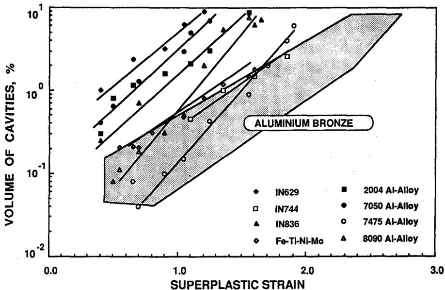
Figure 6. Cavitation behavior of commercial aluminum bronzes, including previously reported results of other superplastic alloys.
