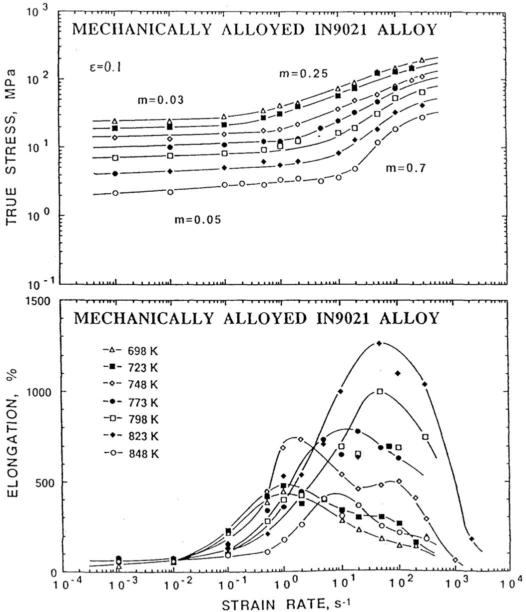
Figure 7. Variation in flow stress (top) and elongation (bottom) for a mechanically alloyed IN9021 aluminum alloy as a function of strain rate for testing temperatures from 698 to 873 K.
