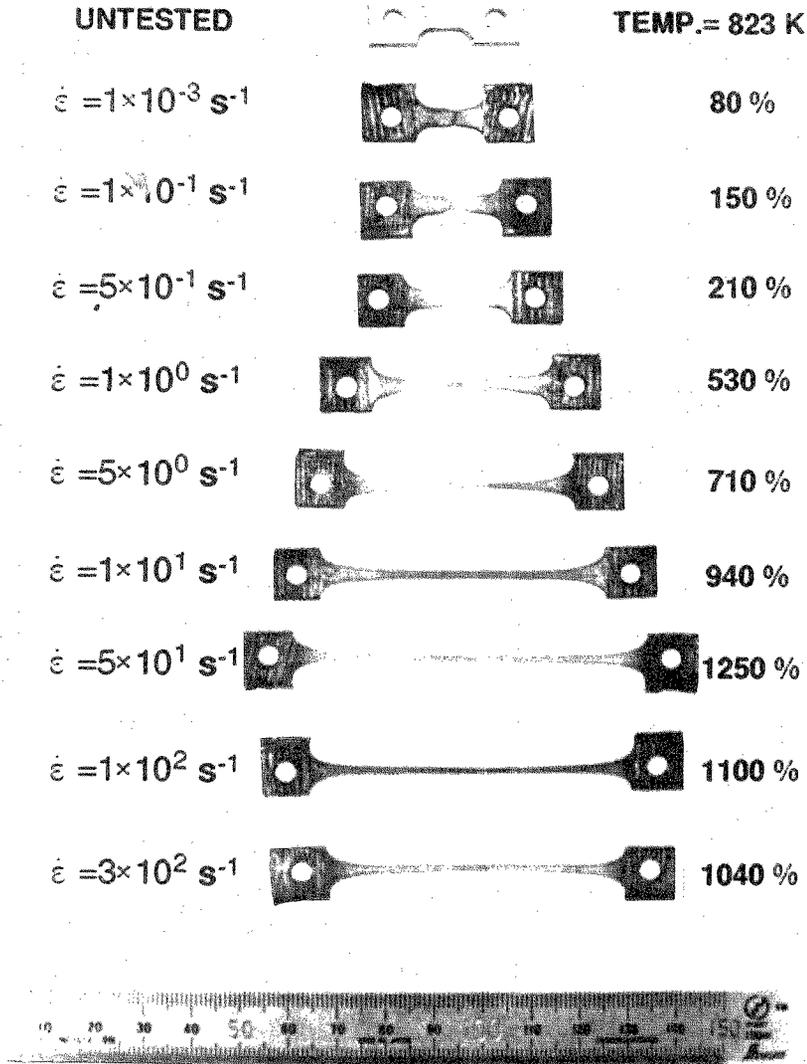
Figure 8. An example of the fractured specimens for the mechanically alloyed IN9021 alloy.
