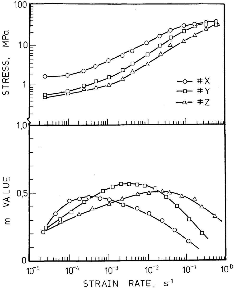
Figure 2. The changes in flow stress and m value with strain rate at a typical superplastic temperature of 1073 K for commercial aluminum bronzes #X, #Y and #Z.
