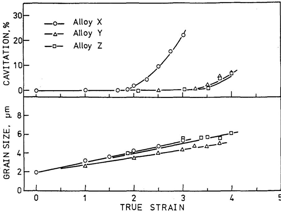
Figure 3. The change of mean size of  $\alpha$ -grains and cavitation behavior of alloys #X, #Y and #Z with strain at 1073 K for the strain rates given in TABLE I.
