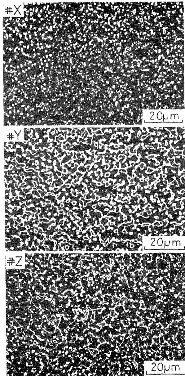
**Figure 1.** Typical superplastic microstructures obtained in the commercial aluminum bronzes #X, #Y and #Z after annealing for 1.8 ks at 1073 K for both alloys #X and #Y, and at 1123 K for alloy #Z.
