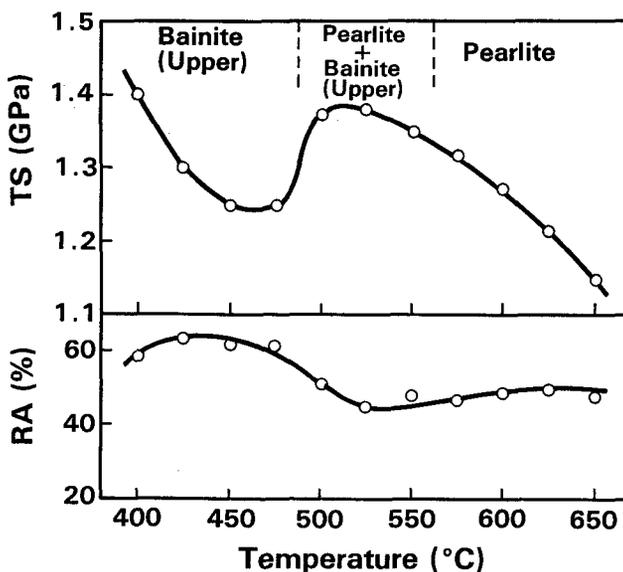
Figure 3. Effect of transformation temperature on microstructure and mechanical properties (Steel F, 0.96C-0.2Cr)
