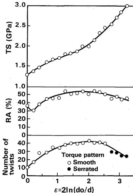
Figure 12. Drawability of Stelmor-cooled wire rod (Steel F, 0.96C-0.2Cr,  $d_0=5.5\text{mm}$ )
