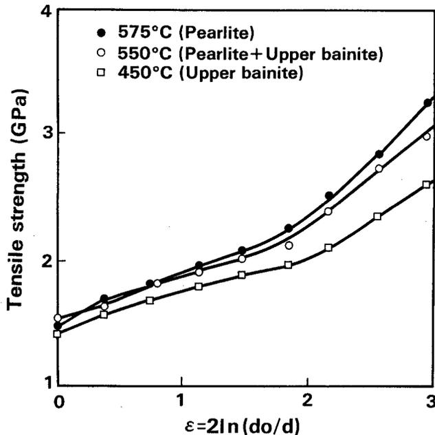
Figure 4. Effect of transformation temperature on work hardening behavior (Steel F, 0.96C-0.2Cr)
