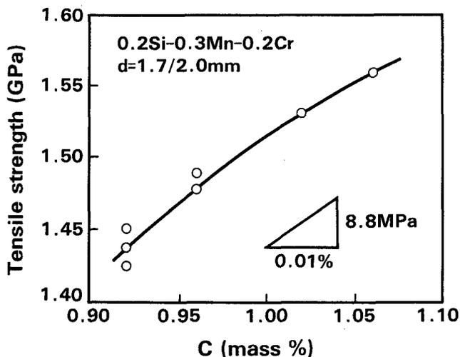
Figure 10. Effect of C content on tensile strength of lead patented wires (LP: 575°C × 12s)
