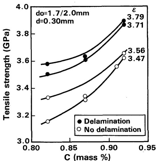
Figure 13. Effect of carbon content on threshold strength of delamination (0.2Si-0.3Mn-0.2Cr, LP: 575°C × 12s)
