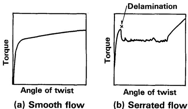
Figure 2. Torque-twist diagrams
