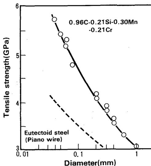
Figure 14. Tensile strength of hypereutectoid steel wire
