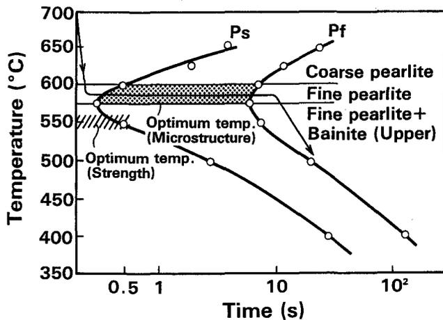
Figure 6. Schematic representation of optimum patenting temperature
