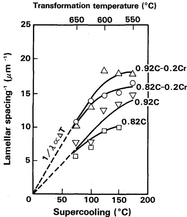
Figure 9. Relationship between pearlite lamellar spacing and transformation temperature
