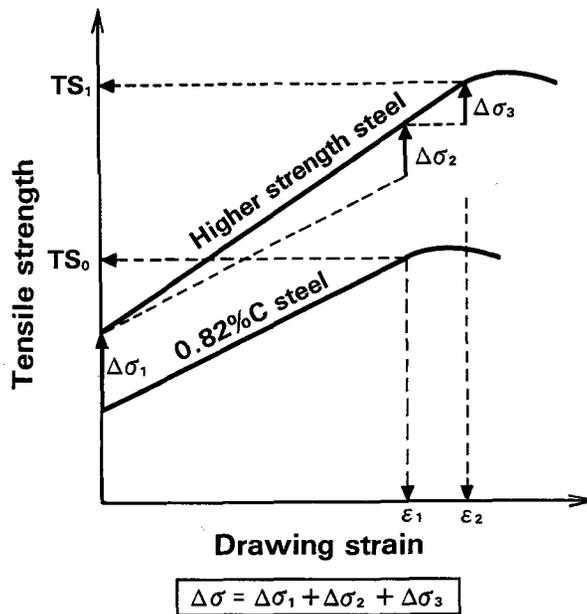
Figure 1. Strengthening of steel wire
