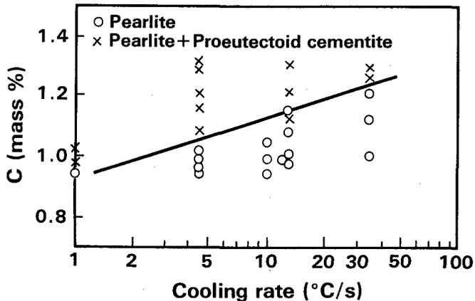
Figure 8. Effects of C content and cooling rate on proeutectoid cementite precipitation in 0.2Si-0.5Mn steel
