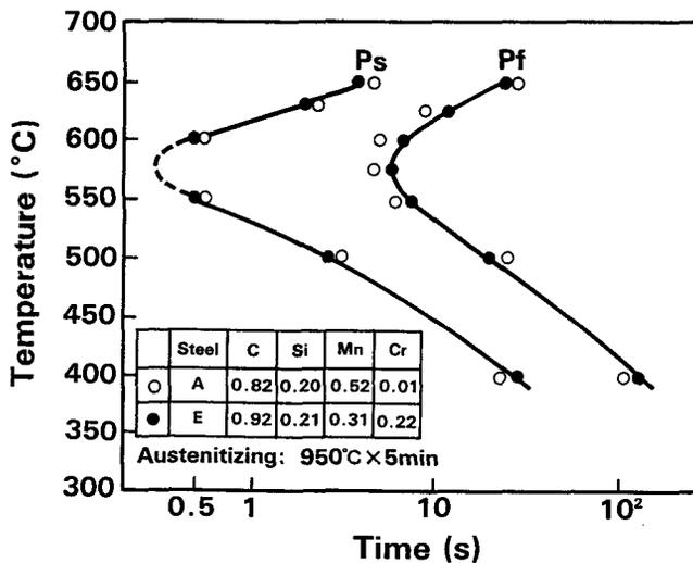
Figure 7. TTT diagram of hypereutectoid steel
