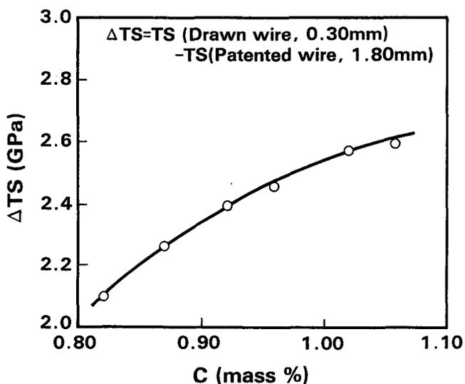
Figure 11. Effect of C content on work hardening of lead patented wires (LP: 575°C × 12s)
