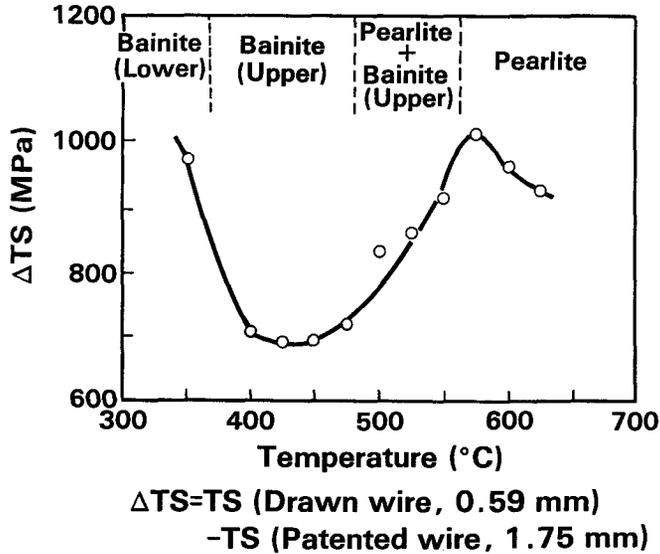
Figure 5. Effect of transformation temperature on work hardening (Steel F, 0.96C-0.2Cr,  $\epsilon=2.17$ )
