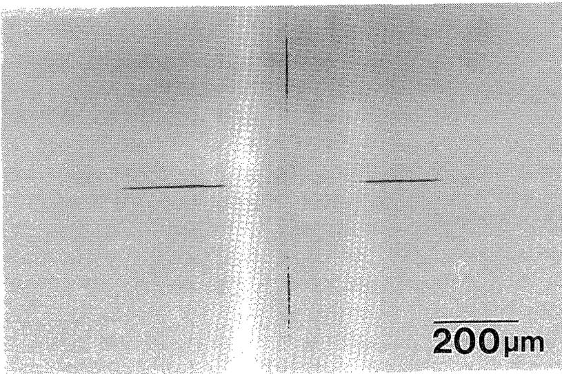
Fig. 3 Optical micrograph of a ground and polished surface after Vickers indentation with an impression load of 50 kgf for Y-TZP.
