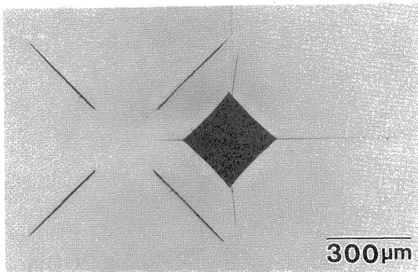
Fig. 5 Crack propagation behavior at around the ground/polished region beneath the indentation for Y-TZP.
