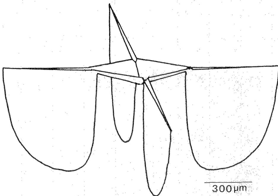
Fig. 4 Schematic drawing of Vickers indentation induced crack in Y-TZP.
