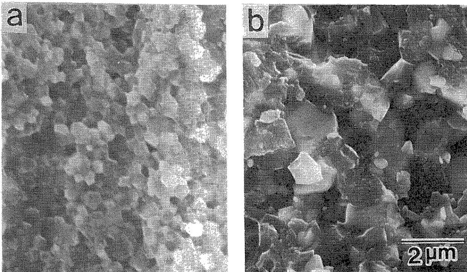
Fig. 1 SEM micrographs of (a)Y-TZP and (b)WC/Y-TZP.
