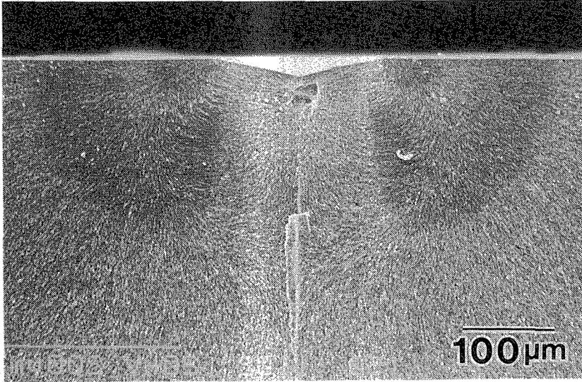
Fig. 2 Fracture surface of Y-TZP showing the crack induced by Vickers indentation.
