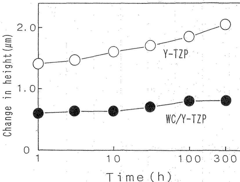
Fig. 8 Relations between protrusion height and aging time at  $150^\circ\text{C}$  for Y-TZP and WC/Y-TZP.
