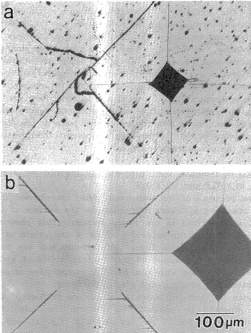
Fig. 6 The same testing results shown in Fig. 5 for alumina (a) and annealed Y-TZP (b). The indented and then polished Y-TZP specimen was heat treated at 1400°C for 30 min before testing.
