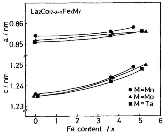
Fig.3 variation in lattice parameter with Fe content of  $\text{La}_2\text{Co}_{17-x-y}\text{Fe}_x\text{M}_y$ .
