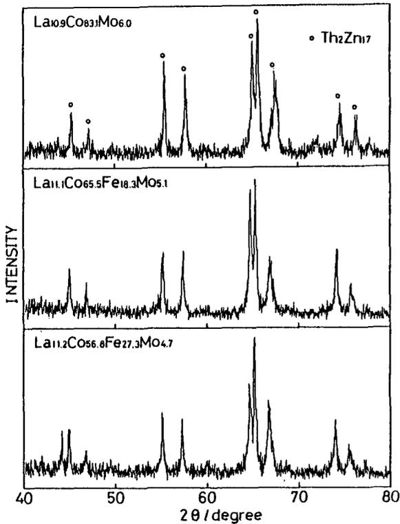
Fig.1 X-ray diffraction pattern of La-(CoFe)-Mo alloys.
