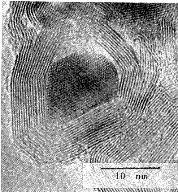
Figure 1. Bright field TEM image of an encapsulated  $\text{CeC}_2$  crystal.
