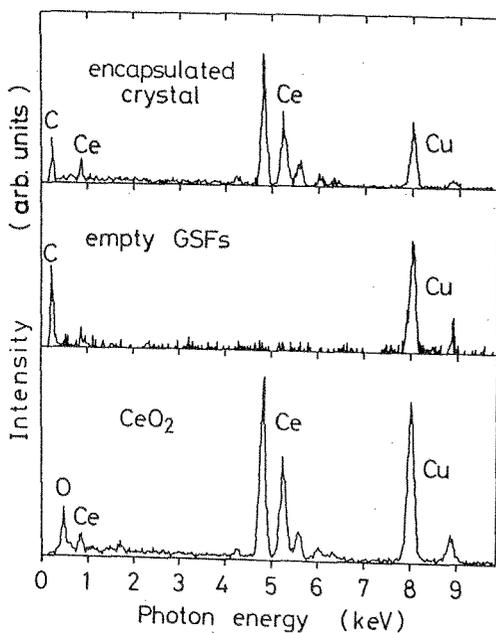
Figure 2. Energy dispersive spectra of an encapsulated crystal, empty GSFs and  $\text{CeO}_2$ .
