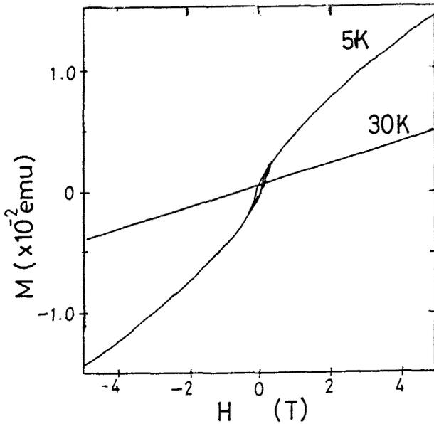
Figure 5 MH curves measured in the wide field range from -5T to 5T at 5K and 30K.
