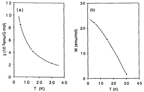
Figure 6 (a) Paramagnetic susceptibility versus temperature. (b) Ferromagnetic saturation moment versus temperature
