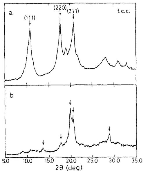
Figure 8 X-ray diffraction charts of (a) the undoped specimen and (b) the specimen doped with IBr.
