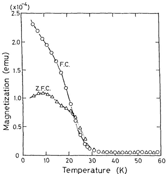
Figure 1 Results of dc magnetization measurements of both ZFC and FC MT curves.
