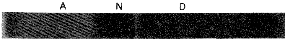
Fig. 2 X-ray topograph showing the distribution of grown-in defects along the cross-section in a FZ-Si crystal with a diameter of 100 mm decorated with Cu. The edge of left hand side is the outer surface and that of right hand side the center of the crystal [13].
