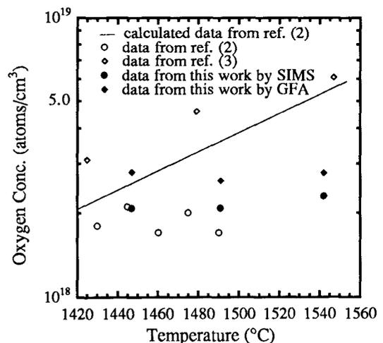
Fig. 2. A comparison of the dependence of oxygen solubility on temperature of undoped silicon melt.
