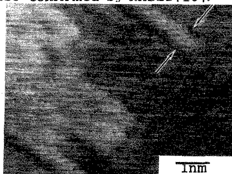
Fig. 2. STM image of epitaxial diamond(001) surface.
