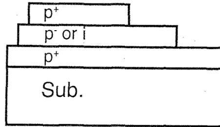
Figure 6. Schematic drawing of selectively grown p-i-p epitaxial trilayered structure.
