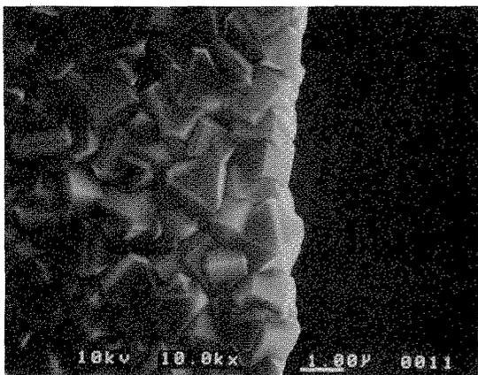
Figure 1. SEM image of selectively grown polycrystalline diamond film.
