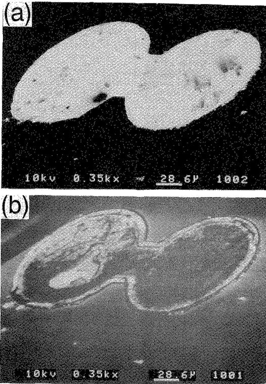
Figure 5. (a) SEM image of selectively grown homoepitaxial diamond film. (b) CL image corresponding to (a). 10 keV.
