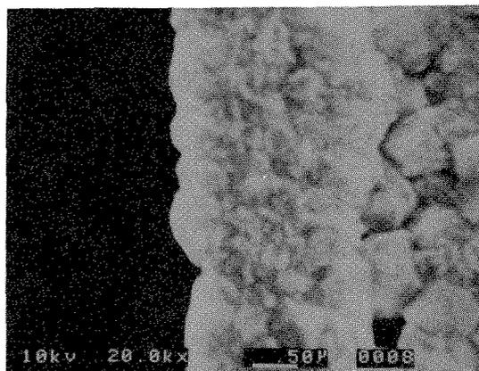
Figure 4. SEM image of selectively grown polycrystalline diamond film.
