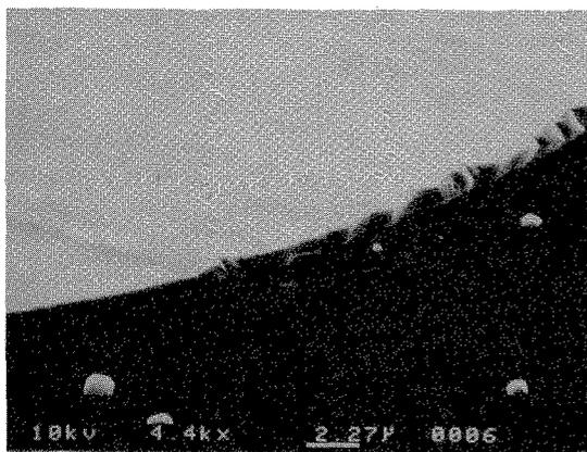
Figure 2. SEM image of selectively grown homoepitaxial diamond film.
