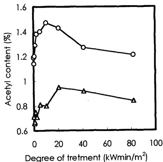
Fig. 1 Effect of degree of corona discharge treatment on acetyl content.
