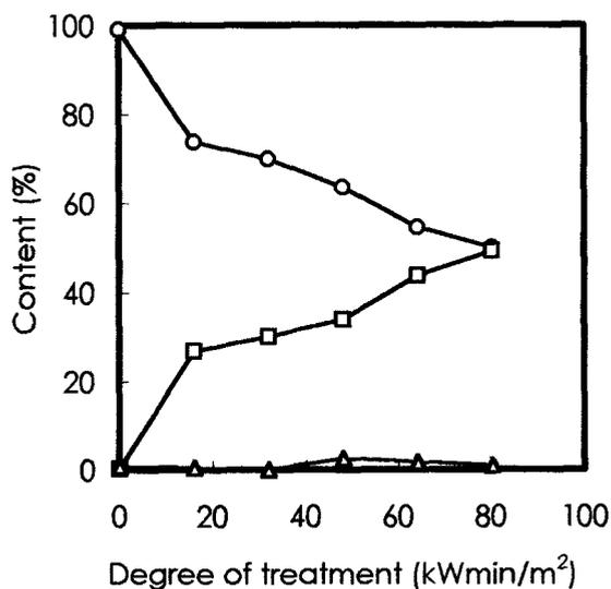
Fig. 3 Effect of corona discharge treatment on  $\alpha, \beta, \gamma$  cellulose content.
