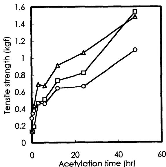
Fig. 5 Effect of acetylation on wet tensile strength.
