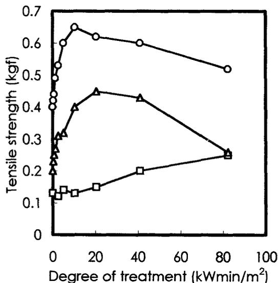
Fig. 2 Effect of corona discharge treatment on wet tensile strength.
