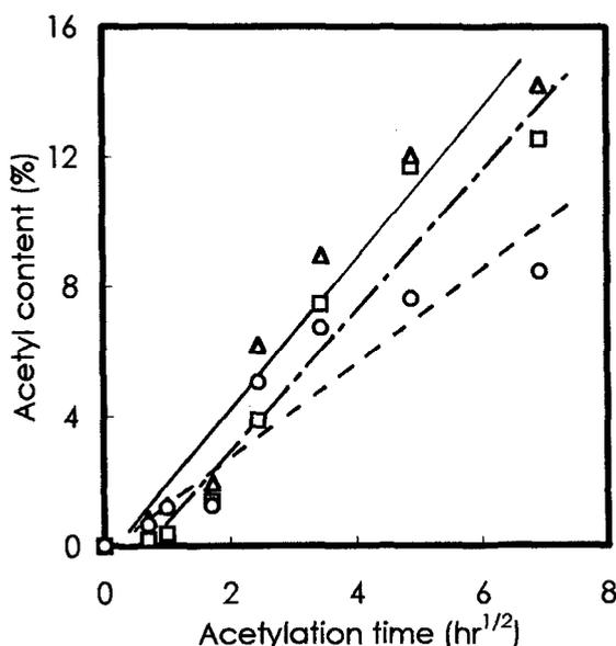
Fig. 4 Effect of corona discharge treatment on acetylation rate.
