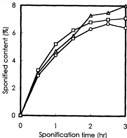
Fig. 6 Effect of corona discharge treatment on saponification of acetylated paper.
