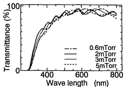
Fig.3. Optical transmittance as a parameter of Ar gas pressure.
