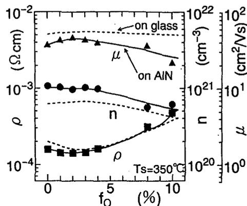
Fig.4. O<sub>2</sub> partial pressure dependence of electrical properties of ITO films. Dashed curves are for on glass substrate.
