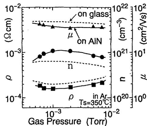
Fig.2. Electrical properties of ITO films prepared on AlN in Ar gas. Dashed curves are for ITO films on glass substrate.
