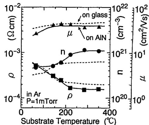
Fig. 8. Substrate temperature dependence of electrical properties of ITO films. Dashed curves are for on glass substrate.
