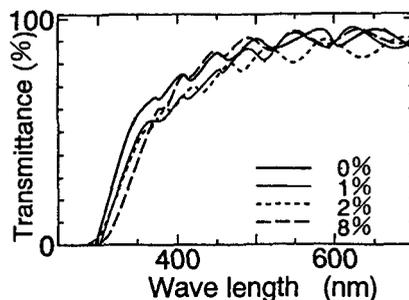
Fig.6. Optical transmittance as a parameter of O<sub>2</sub> partial pressure.
