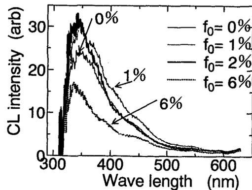
Fig.7. Cathodoluminescence spectra of ITO films on AlN-coated glass substrate.
