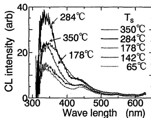
Fig.9. Substrate temperature dependence of cathodoluminescence spectra of ITO films deposited on AlN-coated glass substrate.
