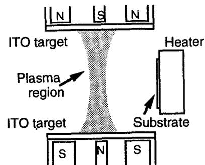
Fig.1. Schematic diagram of facing target sputtering system.
