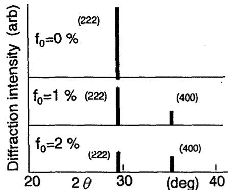
Fig.5. Diffraction patterns as a parameter of oxygen partial pressure.
