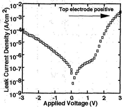
Figure 6. Applied voltage dependence of the leak current density of 3.0μm x 1.4μm x 500
