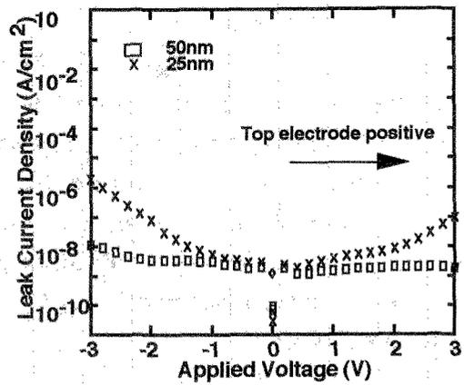
Figure 2. Applied voltage dependence of the leak current density
