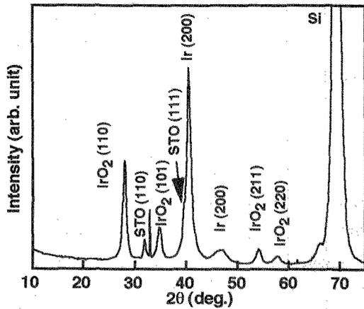
Figure 1. The X-ray diffraction pattern.
