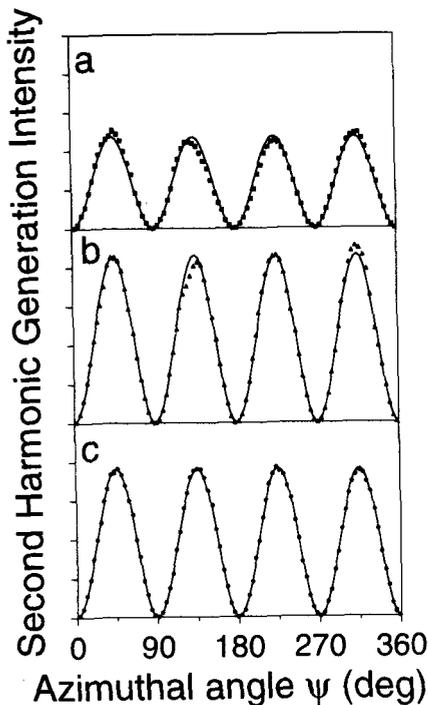
Fig. 2.  $I_{p,s}^{(2\omega)}(\psi)$  from (a) a CuInSe<sub>2</sub> thin film (sample CIS206), (b) a CuGaSe<sub>2</sub> thin film (sample CGS265), and (c) GaAs(001). The data (points) are to scale; the curves are fits using relation (2).
