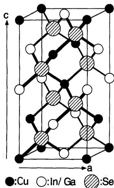
Fig. 1 The chalcopyrite structure.
