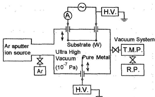
Figure 1 Schematic apparatus of wetting experiment.
