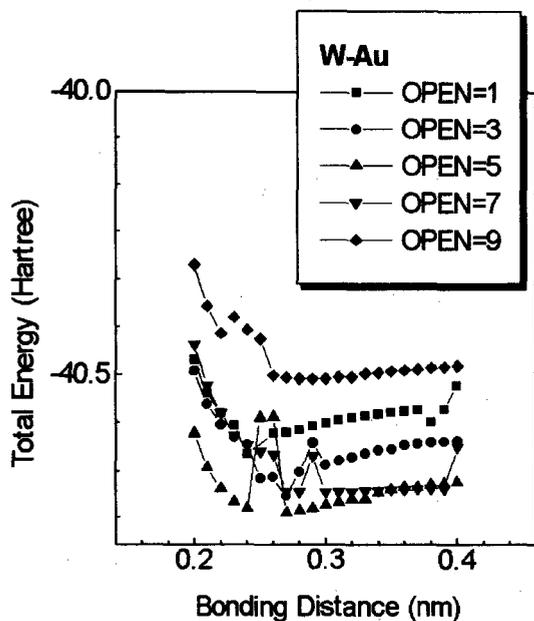
Figure 4 The example of calculated adiabatic potential curves.
