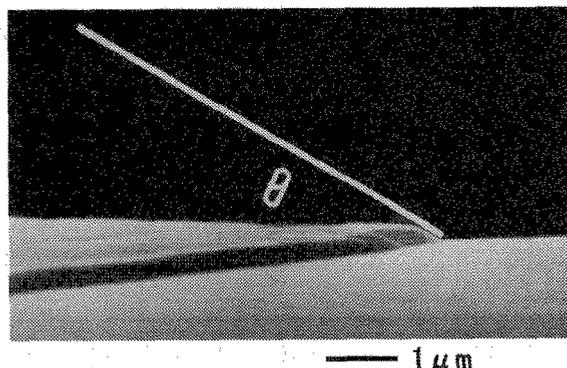
Figure 2 Configuration of measuring of contact angle.
