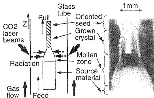
Fig. 1 Schematic of the ILHPG method (left) and side view of the molten zone (right)
