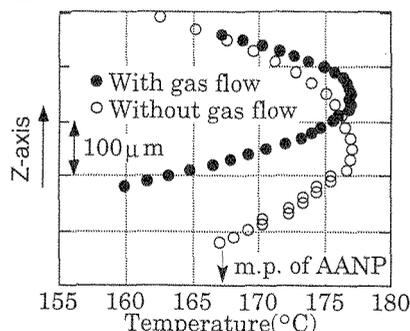
Fig. 3 Temperature gradient in the glass tube. Z-axis is shown in Fig. 1
