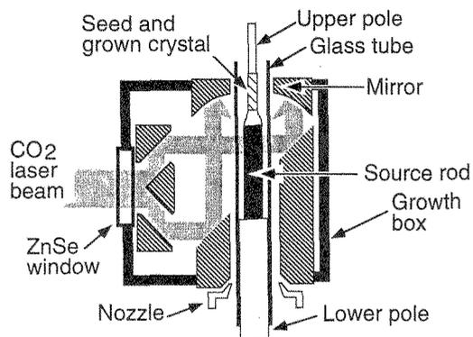
Fig. 2 ILHPG growth apparatus
