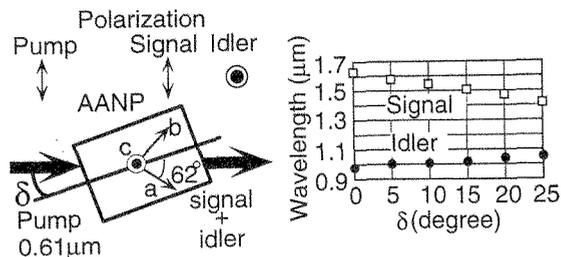
Fig. 5 OPG crystal configuration (left) and wavelength dependence on crystal rotation (right)
