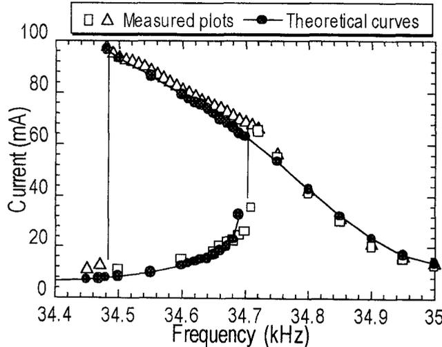
Fig. 7. Theoretical  $\omega$ - $i_0$  curve of the jump phenomena calculated using Eq 9.
