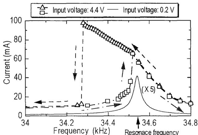
Fig. 2. Frequency response of current around the resonance frequency.
