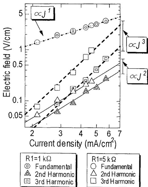
Fig. 3. Fundamental, 2nd, and 3rd harmonic fields as a function of current density at resonance frequency, when  $R_1$  is 1 kΩ and 5 kΩ. The dotted line, solid line, and broken lines are drawn by assuming power law of  $\propto J$ ,  $\propto J^2$ , and  $\propto J^3$ , respectively.
