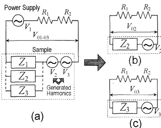
Fig. 4. Equivalent circuits containing the 2nd and 3rd harmonic voltages. (a) is the original circuit. (b) and (c) are circuits only for the 2nd and for the 3rd harmonic voltage, respectively.
