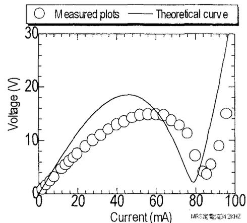
Fig. 6. Theoretical  $v_0$ - $i_0$  curve calculated using Eq 8 at constant frequency 34.2 kHz. The open circles show the experimental values measured with the constant current circuit when  $R_1$  is 5 k $\Omega$ .
