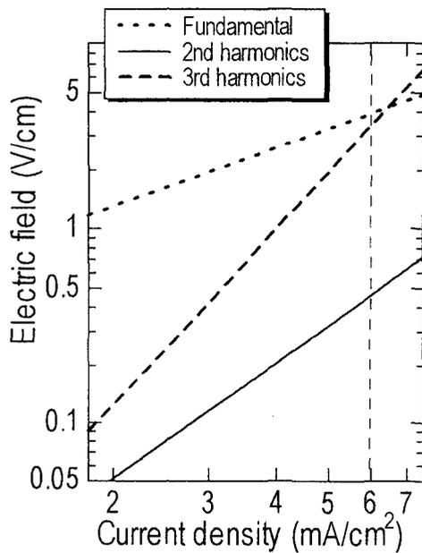
Fig. 5. Fundamental, 2nd, and 3rd harmonic fields corrected using Eq 4 as a function of current density.
