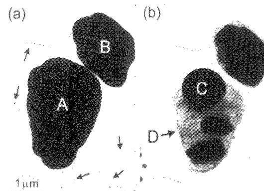
Fig.9 TEM images of compound particles in a  $\text{C}_{60}$ -doped Cu powder mechanically mixed for 128h.
