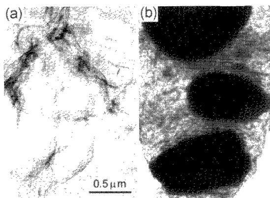
Fig.11 TEM images of compound particles in the  $C_{60}$ -doped Cu powders which were mechanically mixed for (a)2h and (b)128h, respectively.
