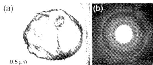
Fig.1 (a)TEM image and (b)EDP of an extraneous substance found in an as-received empty microgrid.
