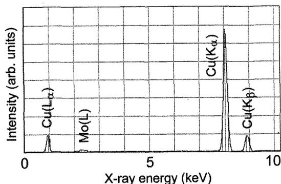
Fig.10 EDX analysis of a compound in a mechanically mixed  $C_{60}$ -doped Cu powder.
