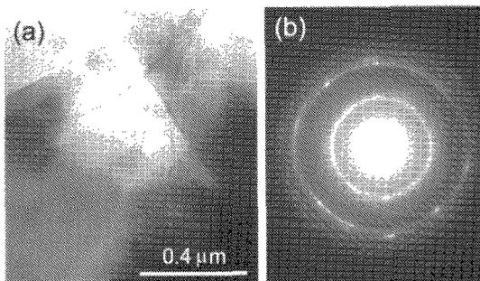
Fig.5 (a)TEM image and (b)EDP of graphite found in a  $C_{60}$ -doped  $ZrO_2$  powder ( $ZrO_2$  - 0.8mass% C) prepared by firing at 500°C for 30 min in air.
