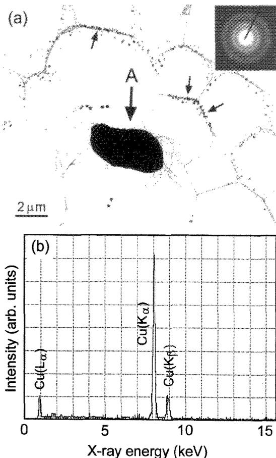
Fig.2 (a) TEM image of an extraneous substance (A) found in an as-received empty microgrid and the diffraction pattern of the tiny particles shown by the smaller arrows. (b) EDX spectrum of the substance A.
