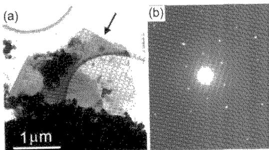
Fig.8 (a)TEM image and (b)EDP of carbyne found in a  $\text{C}_{60}$ -doped  $\text{ZrO}_2$  powder ( $\text{ZrO}_2$ -2mass%C) fired at  $500^\circ\text{C}$  for 30 min in air.
