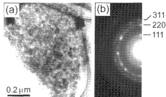
Fig.4 (a)TEM image and (b)EDP of a precipitate of  $C_{60}$  found in a  $C_{60}$ -doped  $ZrO_2$  powder ( $ZrO_2$  - 0.8mass% C) fired at 500°C for 30 min in air.
