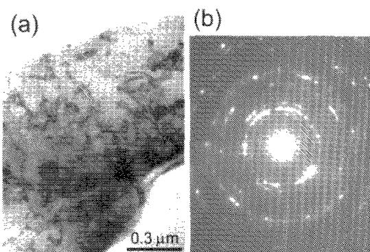
Fig.7 (a)TEM image and (b) EDP of an unknown form of carbon observed in a  $\text{C}_{60}$ -doped  $\text{ZrO}_2$  powder ( $\text{ZrO}_2$ -2mass%C) prepared by firing at  $500^\circ\text{C}$  for 30 min in air.
