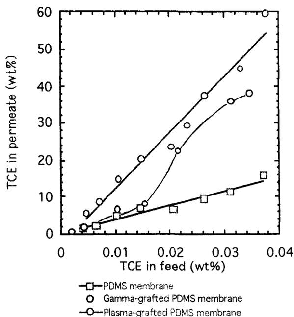
Fig. Pervaporation of TCE/Water mixtures through PDMS membrane and grafted PDMS membranes.
