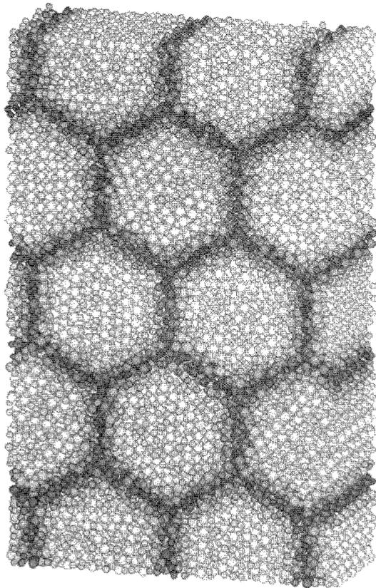
Fig. 1 An example of the simulated polycrystalline sample at 2000 K. The ions are denoted by small spheres, and those having lower coordination numbers are shaded in order to emphasize the grain boundary layers.
