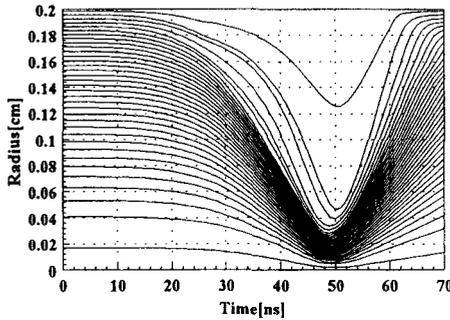
Fig 3 Time-space flow diagram of capillary discharge obtained by 1-D MHD simulation. Radius is represented as a distance from the capillary axis.
