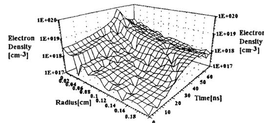
Fig 5 Electron density distributions  $n_e$  of time-space variables in Z-pinch discharge Ar plasma:  $n_e$  in unit of  $\text{cm}^{-3}$ .
