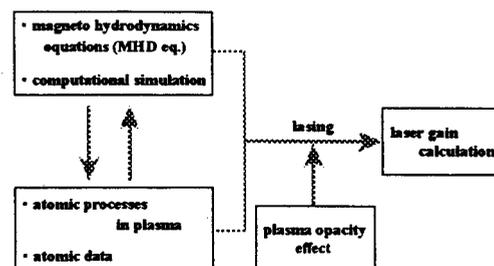
Fig.1 The relation of Z-pinch discharge plasma dynamics considering these plasma atomic processes and application advance of x-ray lasers and soft x-ray source.
