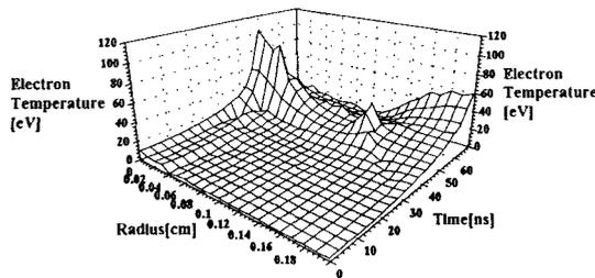
Fig 4 Electron temperature distributions  $T_e$  of time-space variables in Z-pinch discharge Ar plasma:  $T_e$  in unit of eV.
