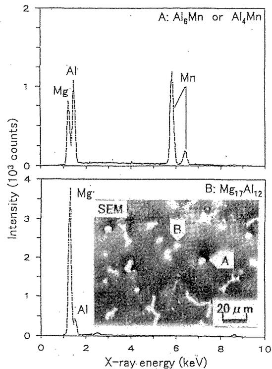
**Fig.4** The results of EDS analyses of the compounds observed in the ingots recycled from the paint-removed professional video camera components.
