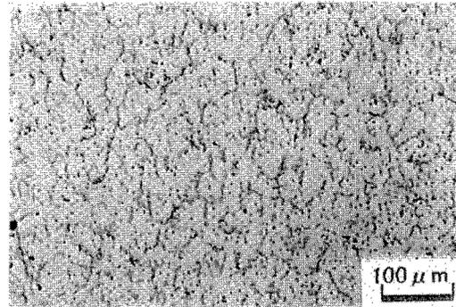
**Fig.3** The microstructures of the ingots recycled from the paint-removed professional video camera components.
