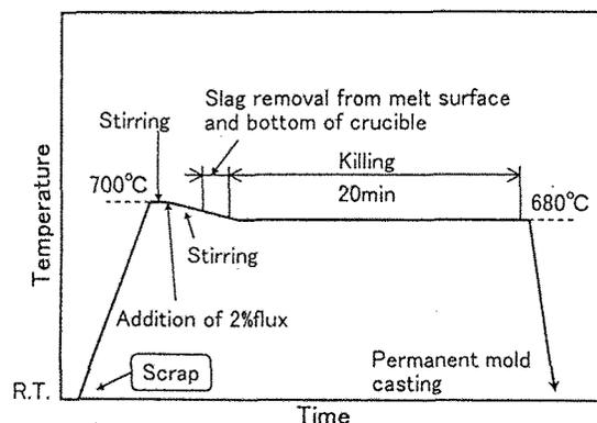
**Fig.1** The schematic diagram of the melting process used in this study.
