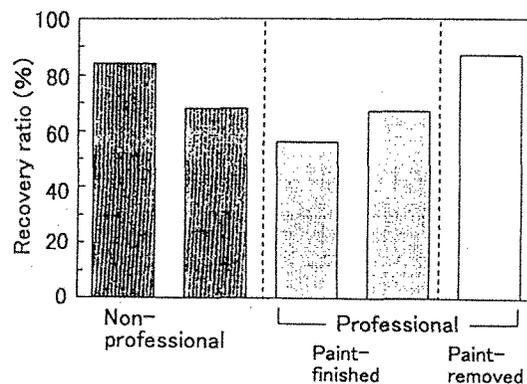
**Fig.2** The recovery ratio of the ingots recycled from the paint-removed professional video camera components compared with that from the professional and non-professional ones with paint finishing.
