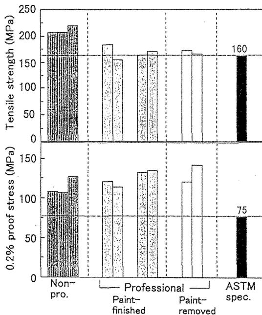
Fig.6 The tensile properties of the specimens recycled from the paint-removed professional video camera components compared with those from professional ones with paint finishing and the non-professional ones.
