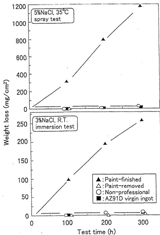
Fig.5 The relationships between test times and weight losses of the specimens recycled from the professional video camera components in comparison with that of AZ91D magnesium alloy virgin ingot and the specimen recycled from the non-professional ones.
