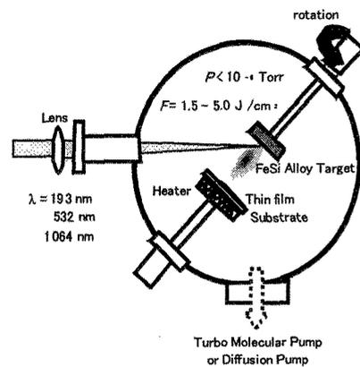
Fig. 1 The experimental schematic for film deposition.
