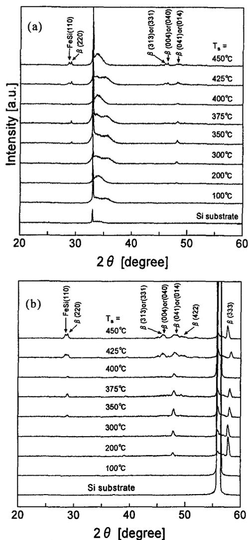
Fig. 3 X-ray diffraction patterns of the films deposited at the various substrate temperature. (a)  $\theta$ - $2\theta$  scan, (b)  $2\theta$  scan (grazing incidence).
