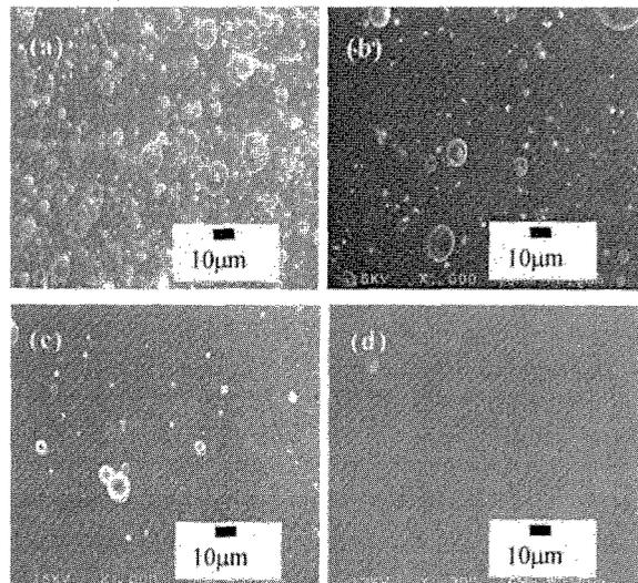
Fig. 2 SEM photographs of the films. (a)  $\lambda = 1064$  nm,  $F = 2$  J/cm<sup>2</sup>, (b)  $\lambda = 532$  nm,  $F = 2$  J/cm<sup>2</sup>, (c)  $\lambda = 193$  nm,  $F = 4$  J/cm<sup>2</sup>, (d)  $\lambda = 193$  nm,  $F = 2$  J/cm<sup>2</sup>.
