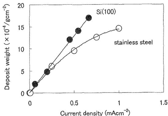
Fig. 3. Relationship between the current density and the deposit weight of the particles on the anode substrates. The sols used for EPD were prepared by reacting an aqueous  $\text{H}_2\text{O}_2$  solution with metallic Sb powder.
