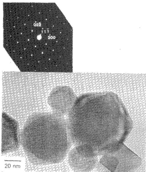
Fig. 1. Bright-field TEM micrograph of the  $\text{Sb}_2\text{O}_5 \cdot n\text{H}_2\text{O}$  particles together with a selected area diffraction pattern. The particles were prepared by a reaction of an aqueous  $\text{H}_2\text{O}_2$  solution and metallic Sb powder at  $\sim 100^\circ\text{C}$  for 1 h.
