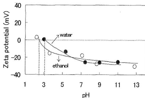
Fig. 2. Zeta potentials of the cubic  $\text{Sb}_2\text{O}_5 \cdot n\text{H}_2\text{O}$  particles plotted as a function of pH. The particles were dispersed in water or in ethanol at a concentration of  $\sim 3 \times 10^{-5}$  M.
