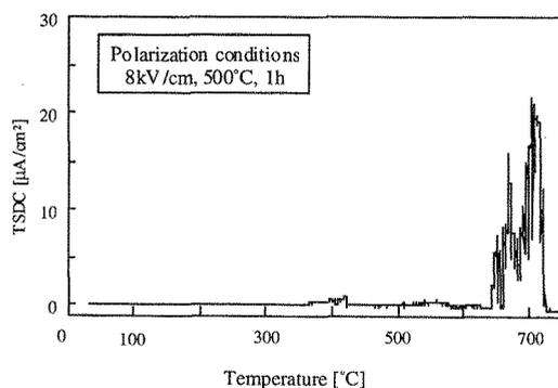
Fig.1 Thermally stimulated current profiles of the HAp ceramics, which was polarized under a dc fields of 8kV/cm at 500°C for 1h, measured at the heating rate 2°C/min.
