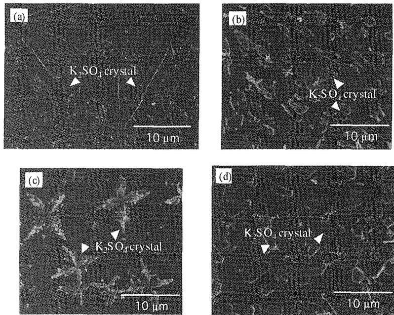
Fig.3 Scanning electron micrographs of  $K_2SO_4$  crystals grown on (a) non-polarized, (b & c) negatively and (d) positively polarized surfaces of the HAp ceramics specimens immersed in the alum+KOH solution with pH=11 for 72h (cooling from 60 to 6°C).
