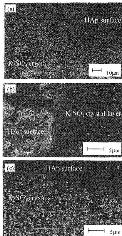
Fig.2 Scanning electron micrographs of (a) non-polarized, (b) negatively and (c) positively polarized surfaces of HAp ceramics specimens immersed in the alum+KOH solution with pH=13 for 24h (cooling from 60 to 6°C).
