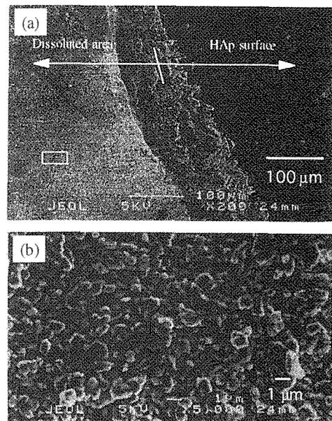
Fig.4 Scanning electron micrographs of non-polarized surfaces of the HAp ceramics specimens after immersed in the Alum solution with pH=3 for 12h (cooling from 60 to 30°C). The enlarged photo (b) is a part of open rectangle in the micrograph (a)
