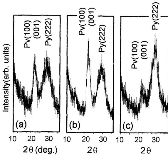
Fig.1 XRD patterns of the PZT films prepared on MgO substrates at (a)400°C, (b)450°C and (c)500°C, respectively, with the heating and cooling rates of 50°Cmin<sup>-1</sup> and the hold time of 0 min.
