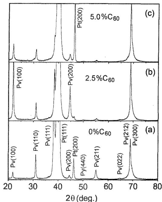
Fig.6 XRD patterns of the PZT films with and without  $C_{60}$  prepared on Pt/Ti/SiO<sub>2</sub>/Si substrates at 500°C.
