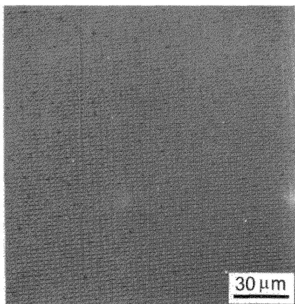
Fig.7 SE image of a  $C_{60}$ -doped PZT film (2.5mass% $C_{60}$ ) prepared on a Pt/Ti/SiO<sub>2</sub>/Si substrate at 400°C.
