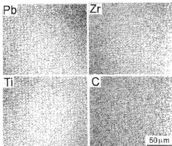
Fig.8 SEM X-ray images of Pb, Zr, Ti and C for the same area as Fig.7.
