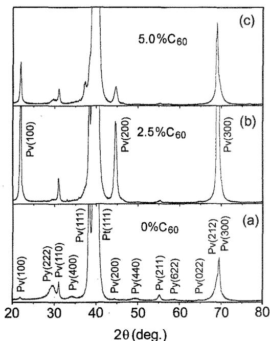
Fig.4 XRD patterns of the PZT films with and without  $C_{60}$  prepared on Pt/Ti/SiO<sub>2</sub>/Si substrates at 400°C.
