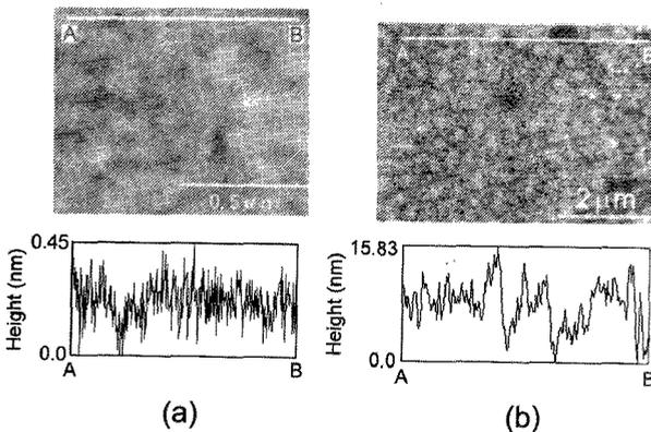
Fig.2 AFM images and surface profiles of the PZT films prepared on MgO substrates at 400°C with the hold time of 0 min (a), and at 600°C with the hold time of 10 min (b), respectively.
