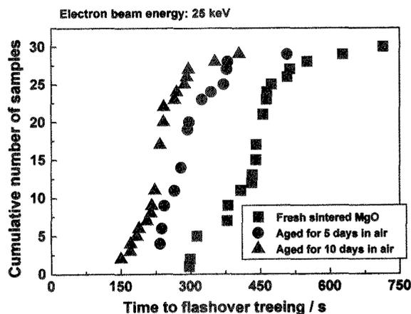
Fig.7. The cumulative number of flashover samples as function of appearance time between the fresh and aged samples.
