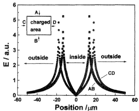
Fig. 4. Calculated shape of electric field distribution on the sample surface bombarded by electron beam. A rectangular area at the surface is the charged area.
