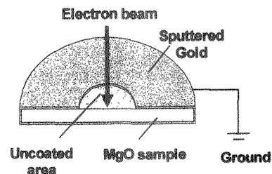
Fig.1. Experimental setup. The electron beam bombarded the center of uncoated area of the sample.
