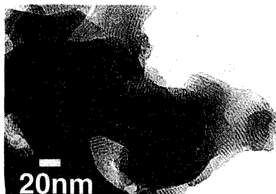
Fig. 3. TEM image of lamellar \text{TiO}_2 after hydrothermal post-treatment (HT) for 24 h at 120^\circ\text{C} .
