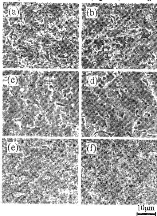
Figure 1 SEM photographs of fractured surfaces of the ceramic samples sintered at 1500°C for (a) 2h, (b) 6h, (c) 12h and (d) 48h, and sintered at (e) 1100°C and (f) 1300°C for 2h.
