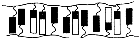
Figure 1. Structure of smectic A phase for ionic P(M6P-IMC- x ): full rectangle, nonionic mesogenic core; open rectangle, ionic azobenzene; full square, ammonium ion.
