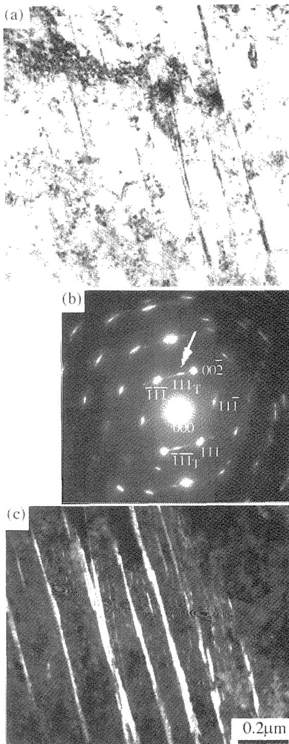
Figure 2. TEM micrographs of the aged sample in 10T at 1013K after being prestrained at room temperature by 35% reduction in diameter. (a) the bright field image, (b) the diffraction pattern, and (c) the dark field image. The dark field image (c) was taken using a diffraction spot,  $[111]_{\tau}$  due to twins, indicated by an arrow in the diffraction pattern (b).
