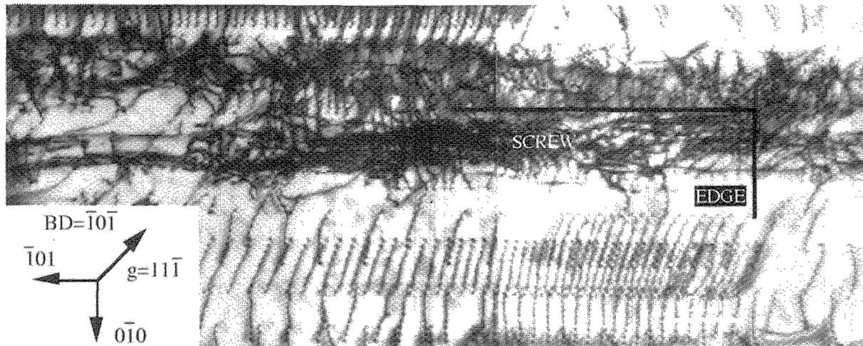
Figure 3 TEM micrograph of the dislocation arrangement in a sample tensile-deformed by 10% at room temperature ( $BD = \bar{1}0\bar{1}$  and  $g=11\bar{1}$ ).
