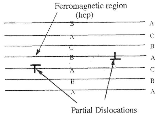
Figure 6 The stacking sequence of close packed (111) planes and stacking fault bounded by the two Shockley partials of a fcc crystal structure.
