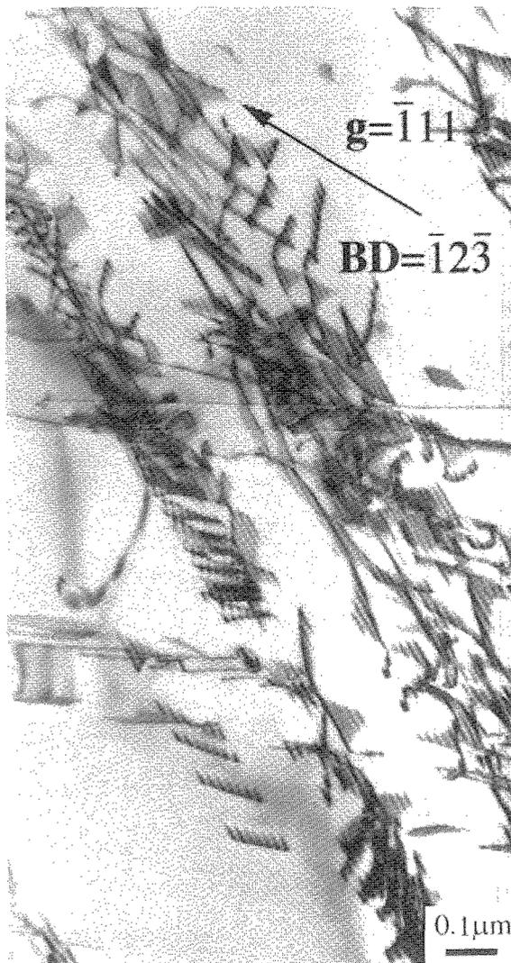
Figure 4. The dislocation structure observed in an aged alloy at 943K for 2h. The specimen was prestrained by 10% in tension at room temperature before the aging treatment. The widely dissociated dislocations having stacking fault fringes are seen in the figure.
