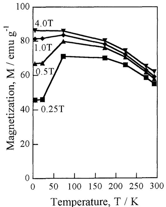
Fig. 3. Saturation magnetization as a function of temperatures for Ni-Mn-Ga-Cu alloy.
