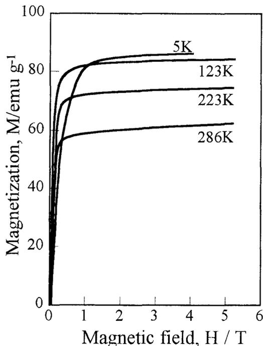
Fig. 2. Magnetization curves obtained at various temperatures for Ni-Mn-Ga-Cu alloy.
