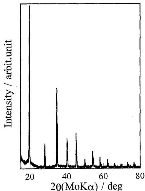
Fig. 1. X-ray diffraction pattern of Ni-Mn-Ga-Cu alloy.
