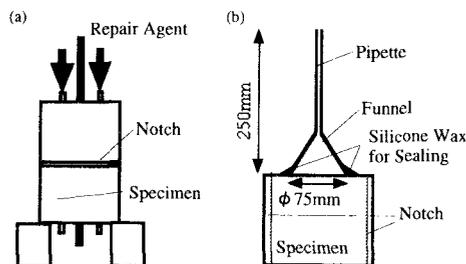
Fig. 7: (a) Repair condition and (b) Test Set-up
