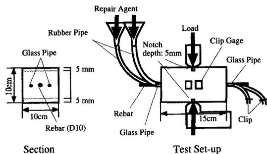
Fig. 6: Test Set-up and Specimen
