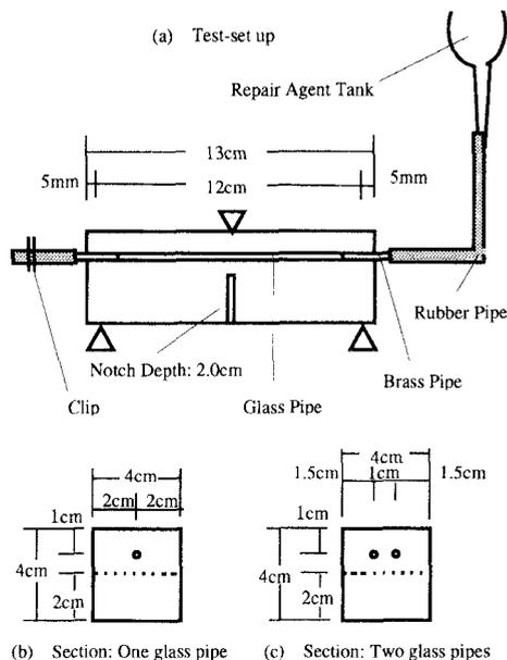
**Fig. 2: Test Set-up and Specimen**
