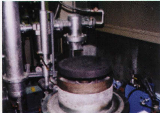
Fig.1 Carbonizing furnace with the rotating specimen table.
