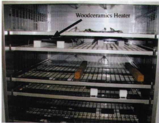
Fig.2 Whole view of the warehouse with the arrangement of woodceramics heater.
