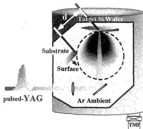
FIG. 1. A schematic of the laser ablation instrument.
