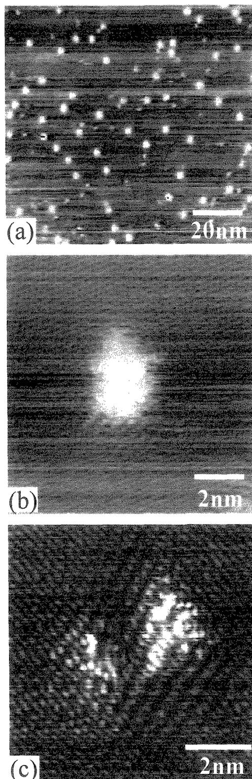
FIG. 2. (a) A typical STM image of the Si nanoparticles deposited on HOPG. (b) A high resolution STM image showing the details of the surface morphology. (c) A Si nanoparticle surrounded by a superlattice structure.
