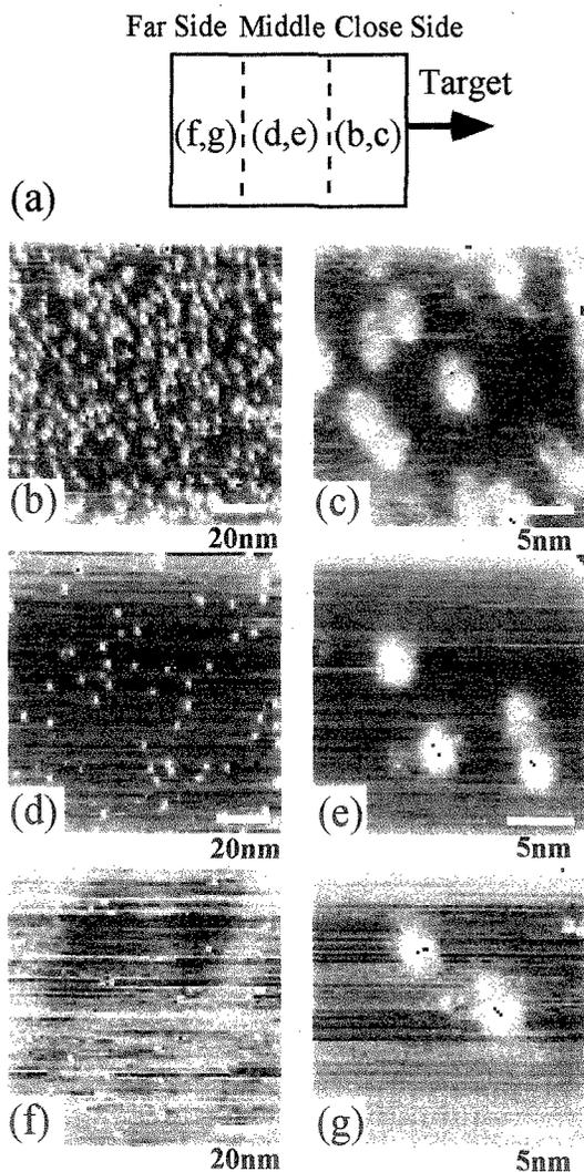
FIG. 3. A set of STM images taken at different locations of the HOPG substrate (both sides and the middle) as indicated in the schematic in (a).
