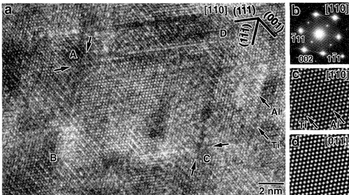
Fig. 2 Defect structure in  $\gamma$ -TiAl crystal irradiated with 15 keV He to a dose of  $8.4 \times 10^{20}$  ions  $\cdot$  m $^{-2}$  at room temperature. a): an HRTEM image of an RD indicated by ABCD; b): an SAD pattern; c) and d): calculated images of  $\gamma$ -TiAl crystals in  $[110]$  and  $[011]$  respectively with defocus of  $-95$  nm.
