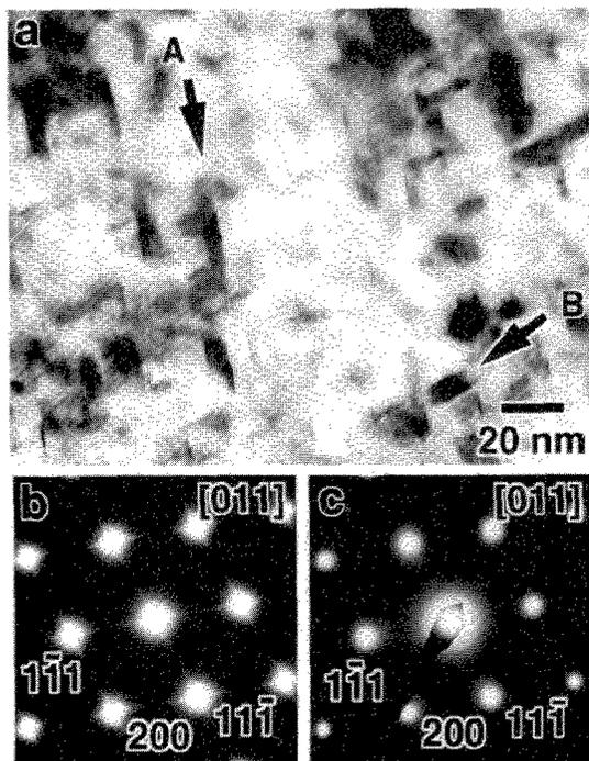
Fig. 1 A micrograph (a) in diffraction contrast (DIFC) mode and a selected area diffraction (SAD) pattern (b) of a  $\gamma$ -TiAl specimen irradiated with 15 keV He to a dose of  $8.6 \times 10^{20}$  ions  $\cdot$  m $^{-2}$  at room temperature.
