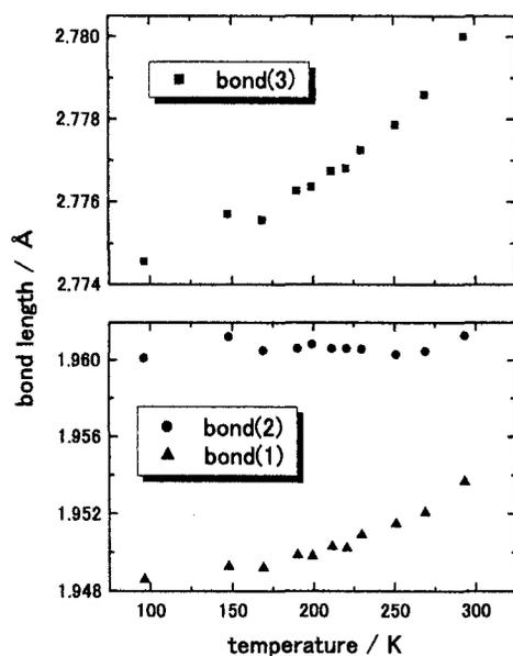
Fig. 3 The temperature dependence of the bond lengths in the  $\text{CuO}_6$  octahedra. The labels (1), (2) and (3) are shown in Fig. 2.
