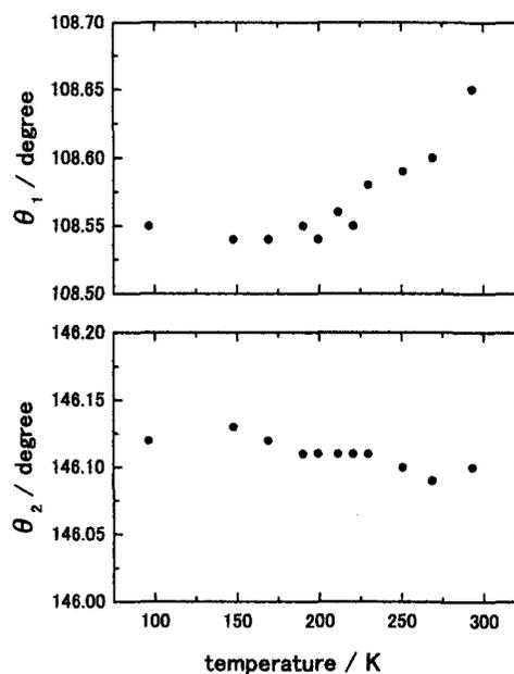
Fig. 4 The temperature dependence of the bond angles  $\theta_1$  and  $\theta_2$ . The angles are defined in Fig. 2.
