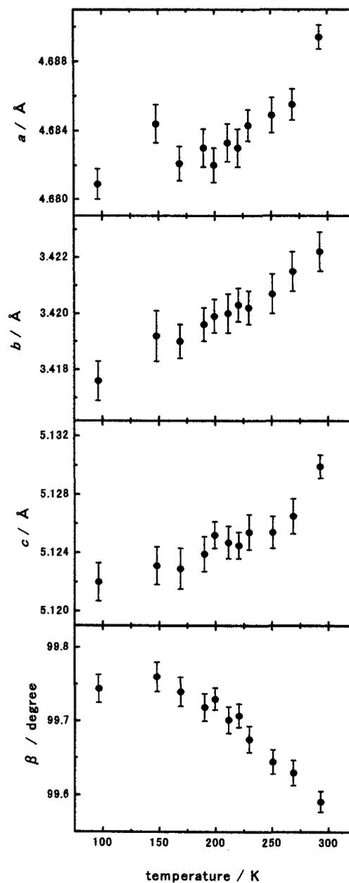
**Fig. 1** The temperature dependence of the lattice constants  $a$ ,  $b$ ,  $c$  and  $\beta$ .
