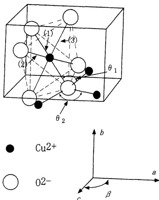
Fig. 2 The distorted octahedral  $\text{CuO}_6$  and the unit cell of  $\text{CuO}$ . The label (1), (2), (3) and  $\theta_1$ ,  $\theta_2$  in the figure indicate the bond lengths and the bond angles between the nearest neighboring atoms, respectively.
