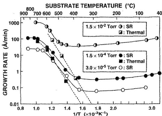
Fig.3 Growth rate of epitaxial Si films as a function of Si substrate temperature. Disilane pressures were  $1.5 \times 10^{-2}$ ,  $1.5 \times 10^{-4}$ , and  $3.0 \times 10^{-5}$  Torr respectively.
