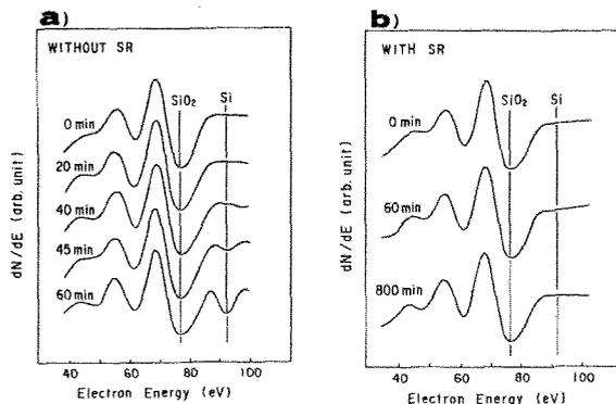
Fig.6 Time dependence of Auger spectra of SiO<sub>2</sub> surfaces obtained after SEG without SR (a) and with SR(b). Surface temperature was 750°C and the disilane pressure was  $3 \times 10^{-5}$  Torr.
