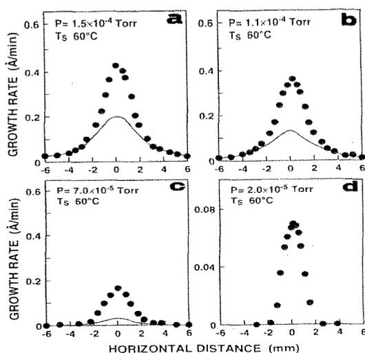
Fig.4 Growth rate distributions on Si substrate as a function of disilane pressure.
