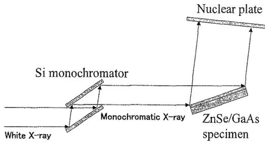
Fig.1 Schematic experimental arrangement of grazing incident X-ray reflection topography.
