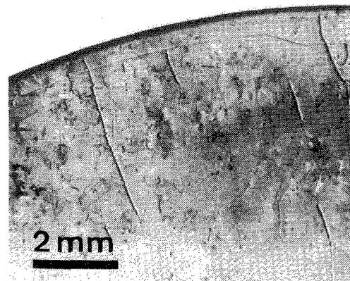
Fig.2 Transmission topograph with white beam X-ray of GaAs substrate.
