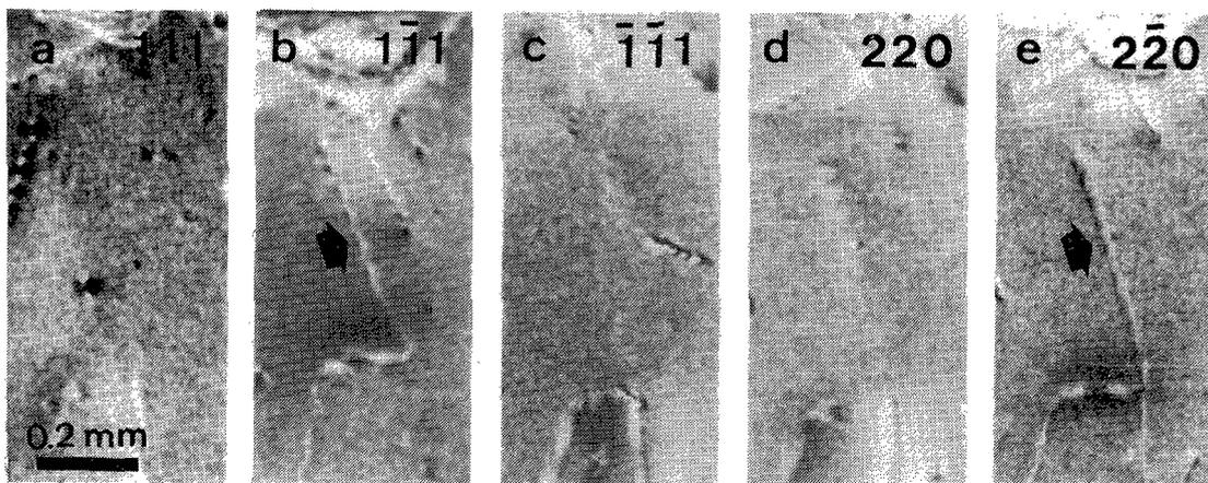
Fig.3 Transmission topographs of GaAs substrate with different diffraction plane.
