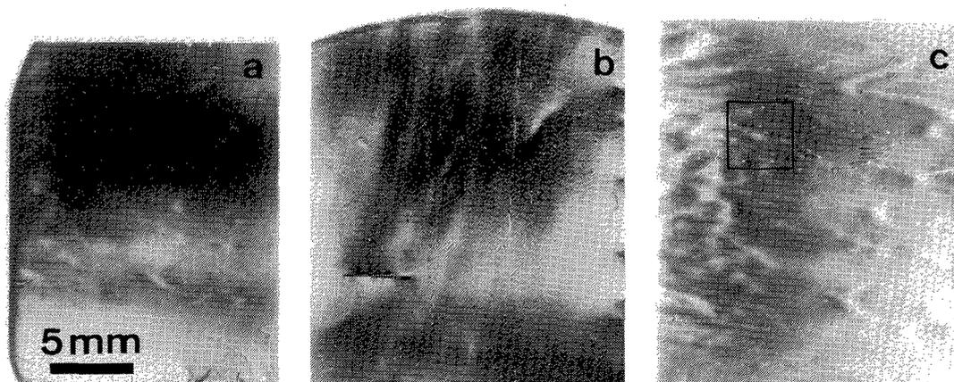
Fig.4 Reflection topographs of ZnSe/GaAs samples with different epilayer thickness.
