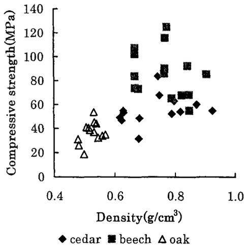
Fig.4 Relationship between compressive strength in longitudinal direction and density of woodceramics.
