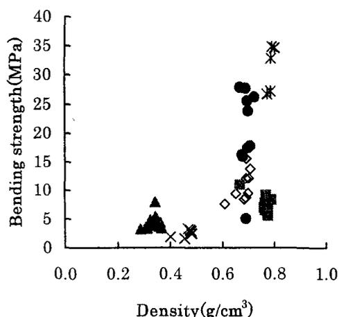
Fig.3 Relationship between bending strength and density of woodceramics.
