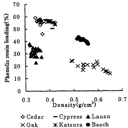
Fig.1 Relationship between phenolic resin loading and density of solid wood.
