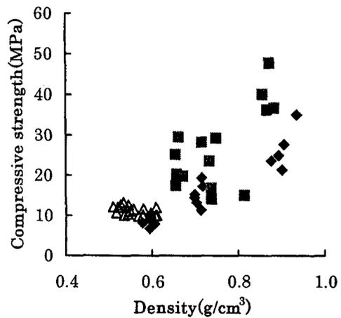
Fig.5 Relationship between compressive strength in radial direction and density of woodceramics.
