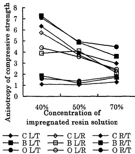
Fig.6 Relationships between anisotropy of compressive strength and concentration of impregnated resin solution.
