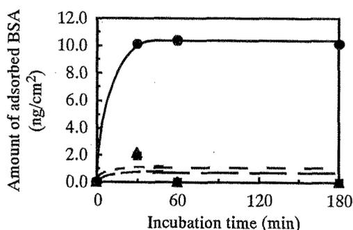
Figure 5 The time dependence of BSA amount adsorbed on the various nanoparticles. Initial concentration of BSA is 20 mg/mL, ●: Polystyrene nanoparticles ( $d = 202$  nm), ▲: PMB30W/PLA nanoparticles prepared in 1.0 mg/mL of PMB30W ( $d = 225$  nm), ■: PMB30W/PLA nanoparticles prepared in 0.1 mg/mL of PMB30W ( $d = 396$  nm).
