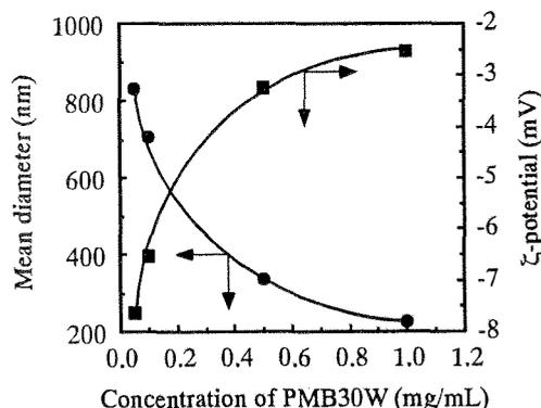
Figure 3 Dependence on the PMB30W concentration of the mean diameter and the  $\zeta$ -potential of PMB30W/PLA nanoparticles. Measurement condition: Solvent: Dulbecco PBS (including 136 mM NaCl) Temperature: room temperature (25 °C).
