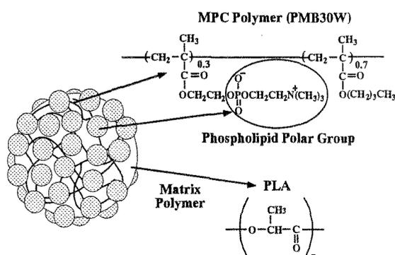
Figure 1 Chemical structure of PMB30W and poly(L-lactic acid) (PLA) and schematic representation of PMB30W/PLA nanoparticles.
